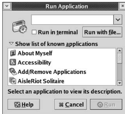
Figure 6-2: The GNOME Run Application dialog box with Show List Of Known Applications selected.
