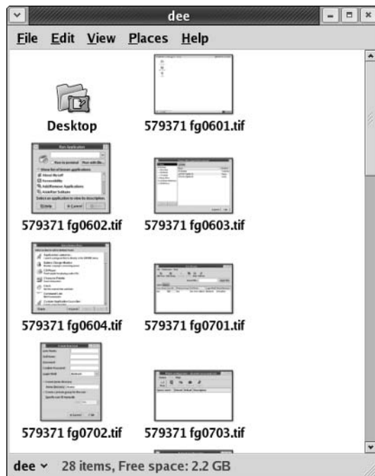
Figure 10-2: Nautilus with the View As Icons option in Dee's home directory in Fedora Core 3.
