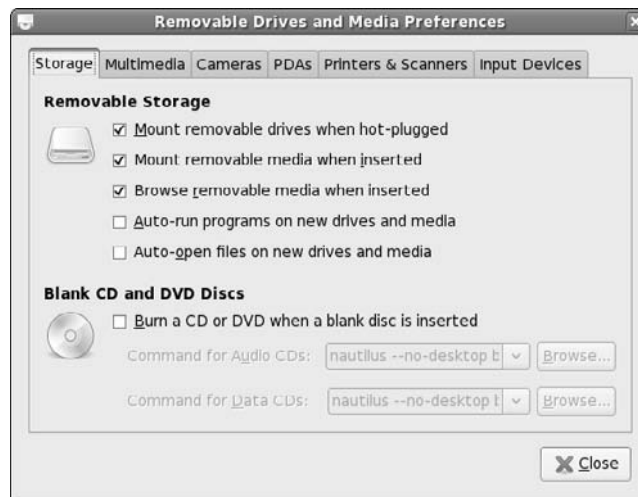
Figure 8-5: The Removable Drives and Media Preferences dialog box with the Storage tab displayed.
