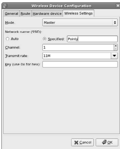
Figure 19-3: The Wireless Device Con- figuration dialog box in the Network Configura- tion tool.
