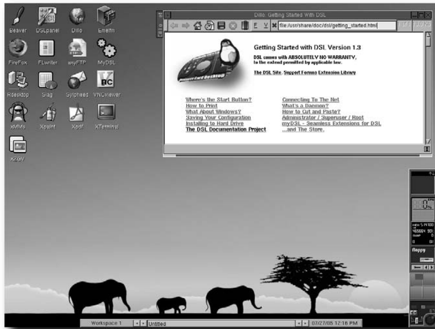
FIGURE 6-3: The Damn Small Linux desktop can boot up directly from a pen drive.
