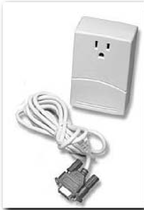
FIGURE 7-4: ActiveHome X10 hardware (CM11A) allows two-way X10 control.
