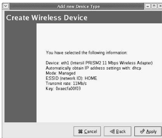
Figure 3-6: Check the information about the wireless connection and click Apply if the information is correct.
