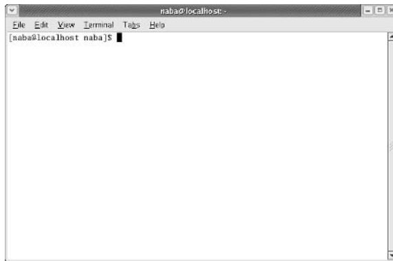
Figure 4-20: You can type Linux commands at the shell prompt in a terminal window.
