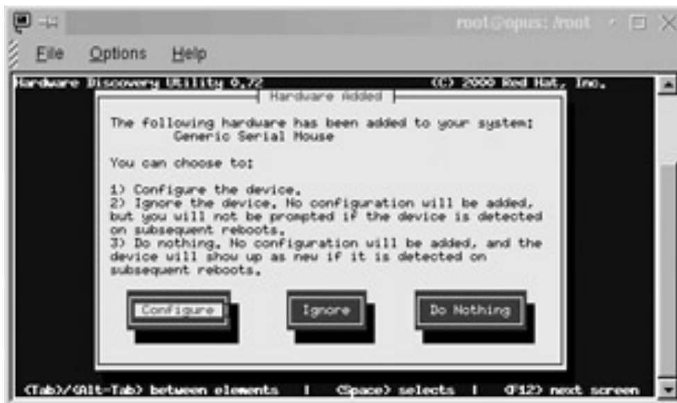
Figure 2.2: The Kudzu utility recognizing a mouse
