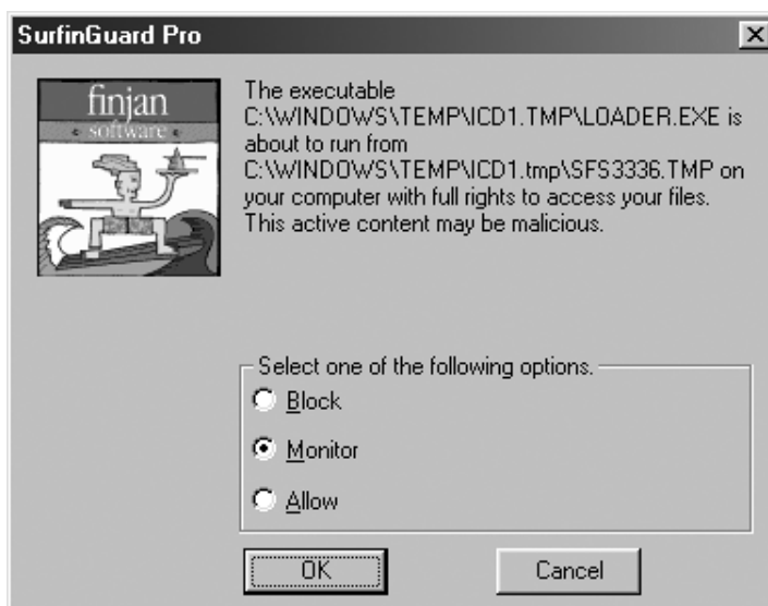
Figure 4.18. SurfingGuard can intercept and block actions taken by suspicious executables.
