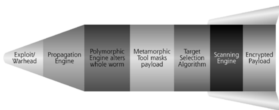
Figure 3.5. Polymorphic and metamorphic components added to the worm mix.
