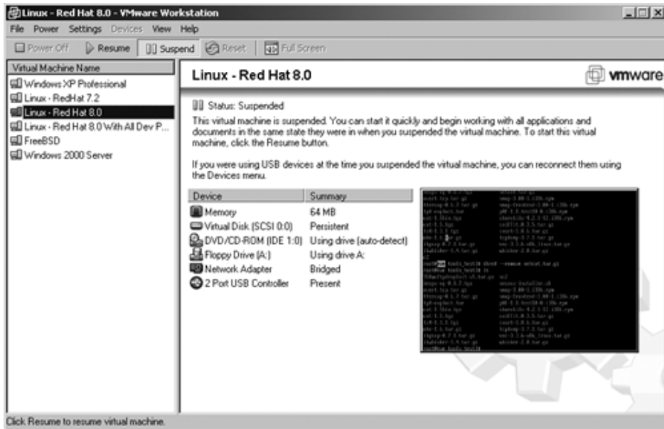
Figure 11.3. My malware analysis laboratory, implemented on a single physical machine, with VMWare.
