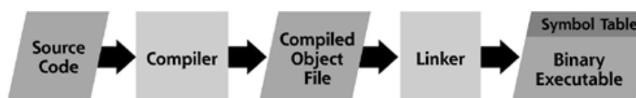
Figure 11.6. Going from source code to binary executable
