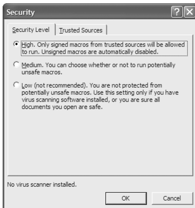
Figure 2.12. Microsoft Office processes macros according to the security level established by the user.
