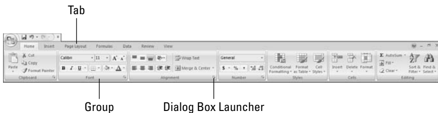
Figure 1-3: Excel's Ribbon consists of a series of tabs containing command buttons arranged into different groups.
