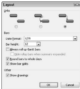
Figure 2-12: Use this dialog box to change layout characteristics for Gantt Chart view.
