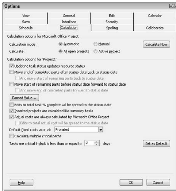
Figure 3-5: Click the Earned Value button to select a method to calculate Earned Value.
