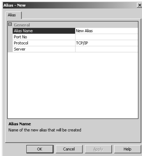
Figure 9-17 Alias – New window used to create a new SQL Server 2005 server alias.
