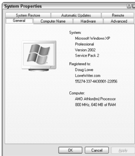
Figure 1-2: The System Properties dialog box shows the Windows version and the amount of RAM installed on the computer.
