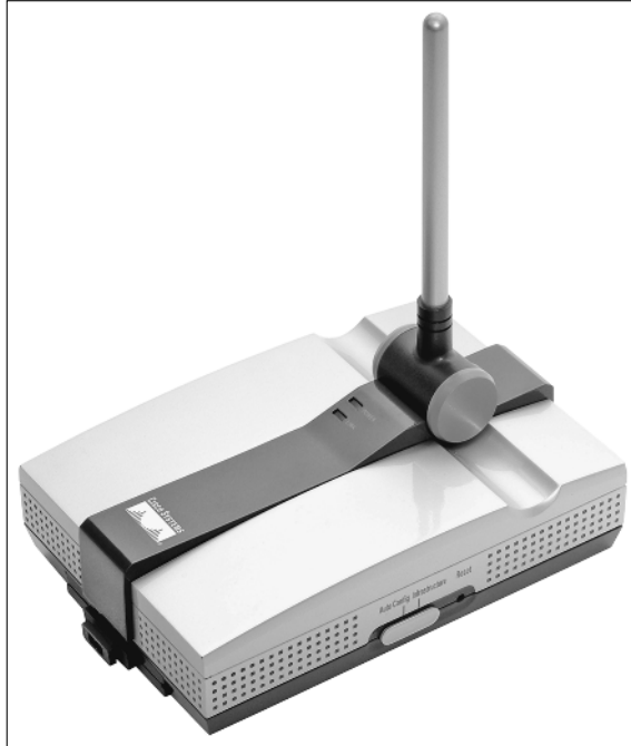
Figure 4-2: A wireless repeater such as this one from Linksys can help increase the range of your wireless network.
