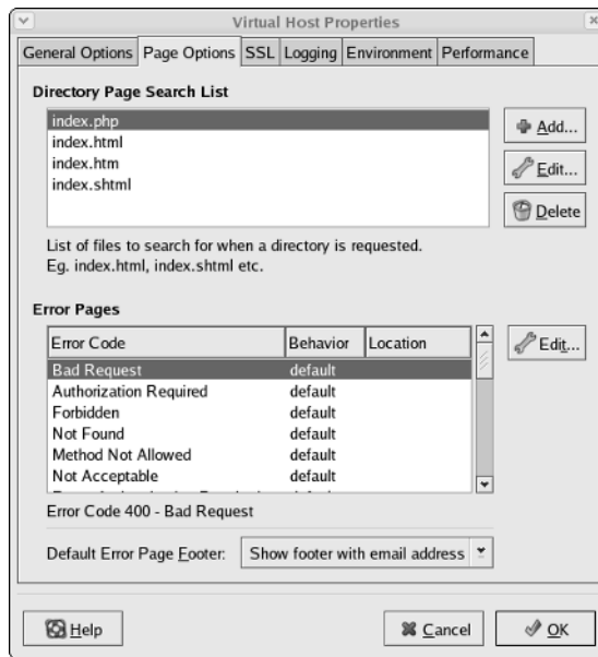
Figure 6-7: The Page Options tab lets you set the directory search list and custom error pages.
