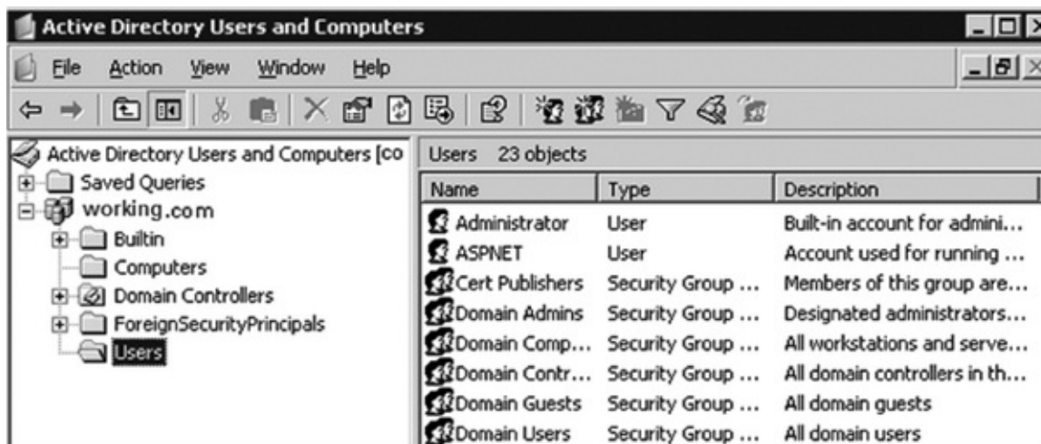
Figure 23-2 You use an Active Directory Users And Computers dialog box like this one to create ACEs for Windows objects.
