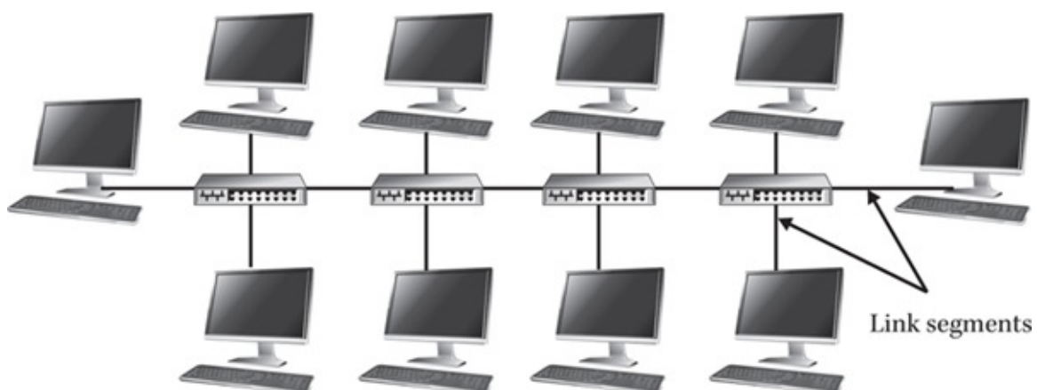
Figure 10-5 Twisted-pair networks use link segments to connect to the computers, making it possible to have four populated hubs.
