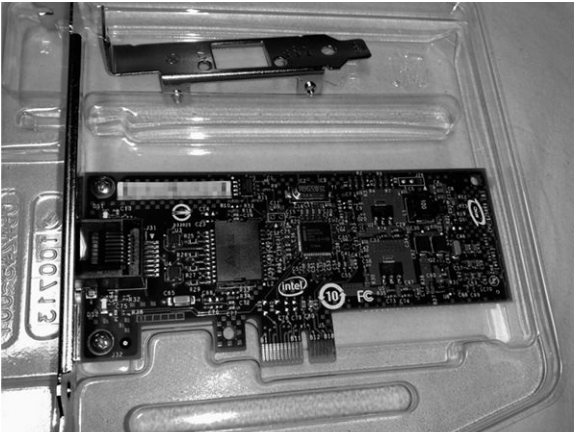
Figure 3-1 A typical Ethernet network card (photo provided by Dsimic at English Wikipedia under the GNU Free Documentation License)
