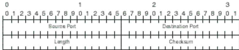
Figure 4.2 The format of the UDP header.
