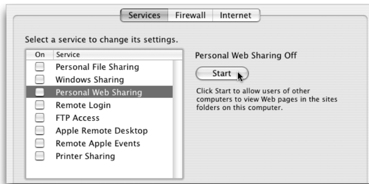
Figure 2-6. The Apache web server on a Mac is switched on and off in the Sharing section of System Preferences.
