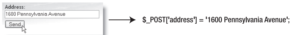
Figure 3-4. You can retrieve the values of user input through the $_POST array, which is created automatically when a form is submitted using the post method.
