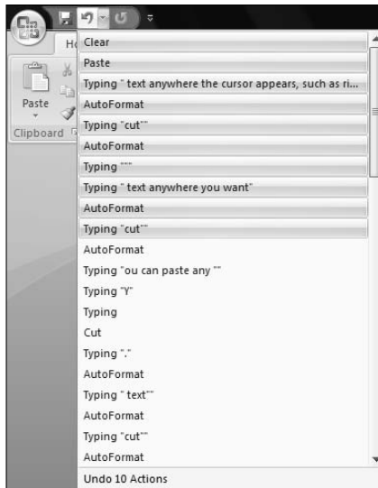
Figure 2-7: The downward-pointing arrow to the right of the Undo icon lets you view a list of your last commands.
