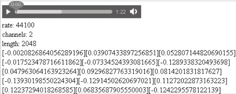
FIGURE 11.2 The audio file's framebuffer data shown onscreen as the audio is being played.
