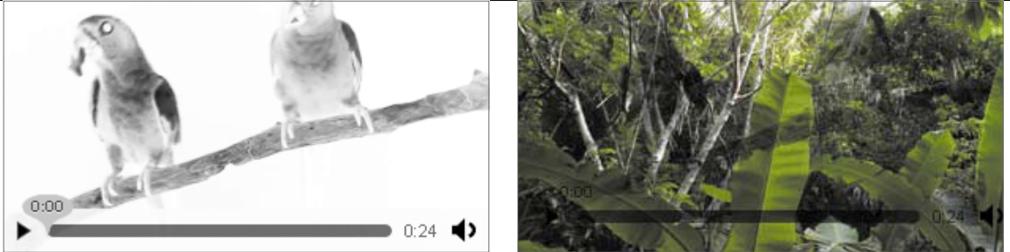
FIGURE 10.13 The video with the luminanceToAlpha colour matrix type applied to it (left). The large white areas are transparent, and a background image would show through them, as shown on the right, where you can barely make out the parrots and the branch.
