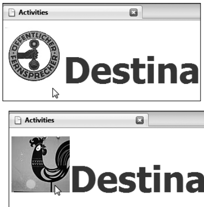
Figure 9.26 An image swap behavior as tested in the browser: The first image appears (top) before the cursor rolls over the area, triggering a swap to the second image (bottom).
