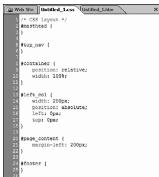
Figure 8.17 In the CSS file, only three of the six ID names (#container, #left_col, and #page_content) start off with positioning properties.
