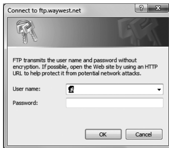
Figure 12.19 When the Connect to dialog box appears, enter the user name and password assigned to you by the ISP or the server's administrator.
