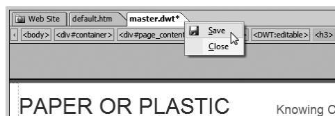
Figure 2.15 Right-click the tab of the .dwt (master) page, and choose Save from the drop-down menu.
