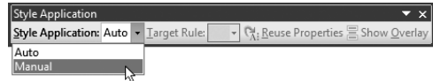
Figure 1.3 The Style Application, normally set to Auto, can be switched to Manual using the toolbar’s drop-down menu.
