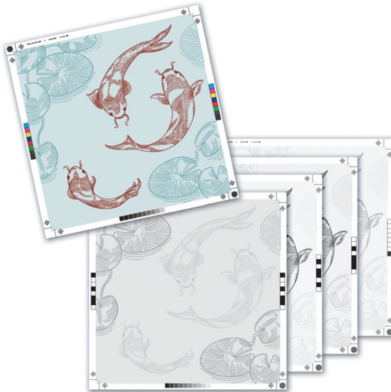
Figure 15.6 Printing a composite is perfect for proofing (top). Printing separations is required for printing colors on a printing press (four underlying pages).
