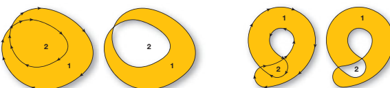
Figure 3.31 Some compound paths appear different, depending on the fill rule specified, especially with self-intersecting paths.
