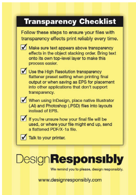
Figure 15.22 The transparency checklist offers a few quick reminders to help ensure your file prints correctly.
