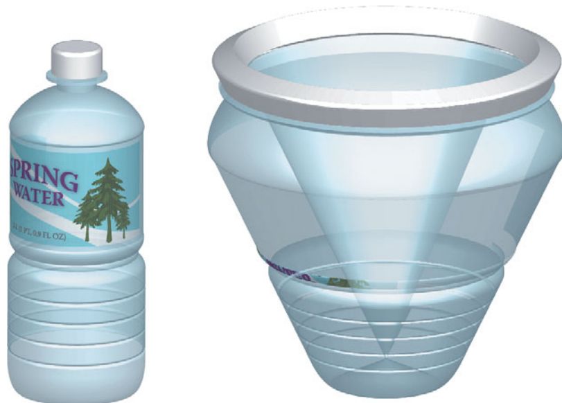
Figure 11.12 What started as a water bottle (left) may not appear the same when you rotate it on the artboard (right). To rotate the bottle in 3D, you have to edit the 3D effect.
