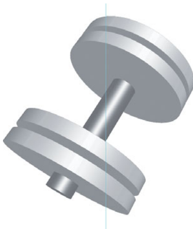
Figure 11.45 Adding a Perspective setting can add a touch of realism to your barbell. Try adding more lights and increasing the highlight intensity and blend steps to get a more metallic look.
