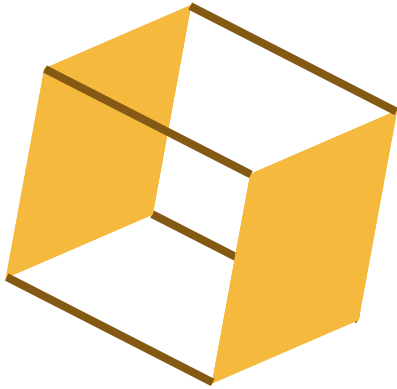
Figure 11.21 A normal extrude is created by connecting the front and back faces of an object with a straight line.
