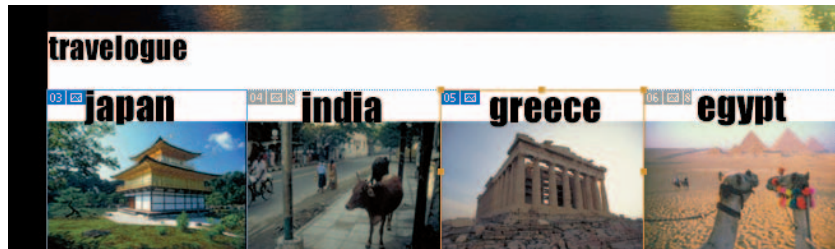
Figure 2-2: A solid selection box and number appears when you slice your image.
