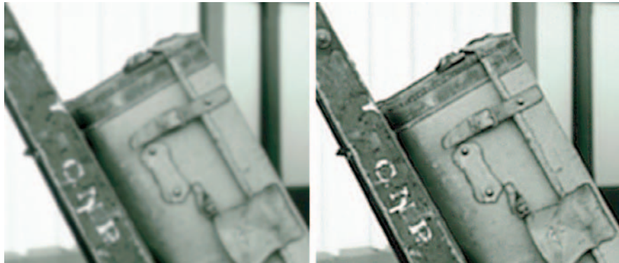
Figure 1-5: Sharpening an image boosts the contrast of neighboring pixels and gives the illusion of improved focus.
