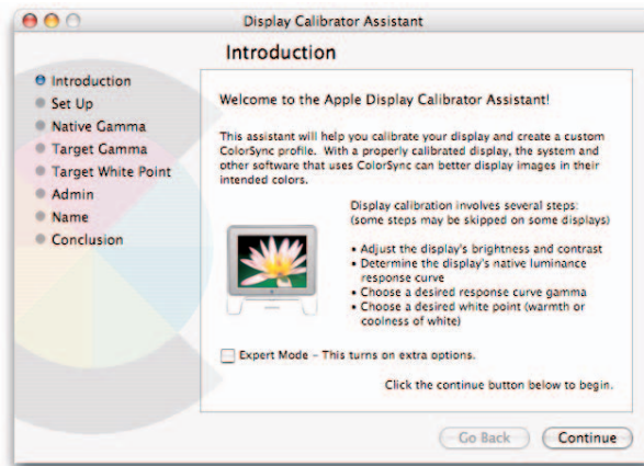
Figure 3-7: Mac users can use the Display Calibrator Assistant to calibrate their monitors.
