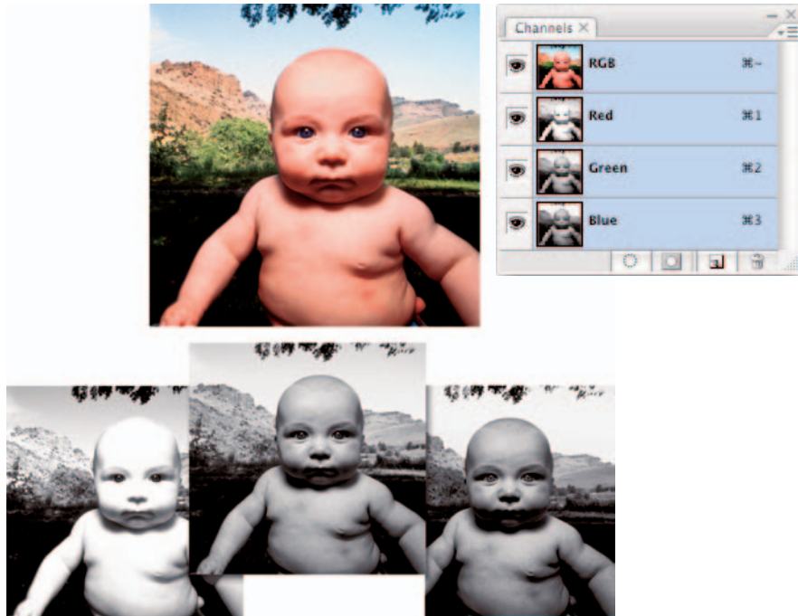
Figure 1-1: A color image is composed of 8-bit grayscale images referred to as channels.
