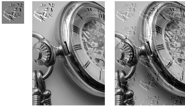
Figure 8.3 Watermarks added to an image by modulating it with an embossed logo (far left), using Image::Magick . The image in the middle was produced with the opacity set to 60 percent and the gravity to NorthWest , and the one on the right was produced with an opacity of 25 percent and the tile option.
