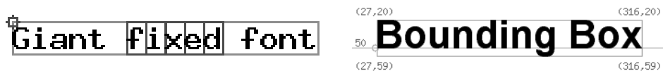
Figure 11.1 The size parameters and handles for strings with GD . For fixed-width fonts, the only parameters of importance are the width and height of the single characters and the handle is located at the upper-left corner of the string. For TrueType fonts, the parameters of importance consist of the coordinates of the bounding box around the whole string to be drawn, and the handle is located at the baseline of the font.
