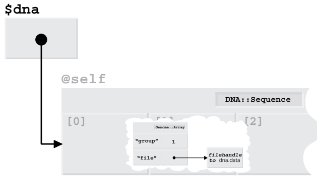
Figure 9.6 Internal structure of a DNA::Sequence object
