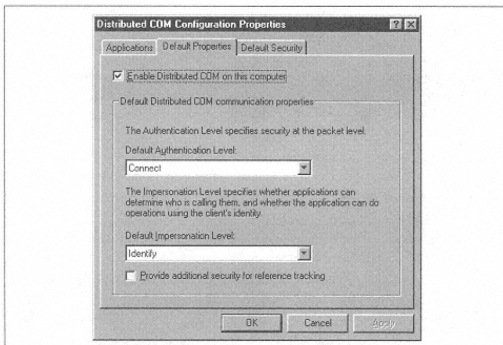
Figure 12-5. DCOM configuration tool with DCOM enabled
