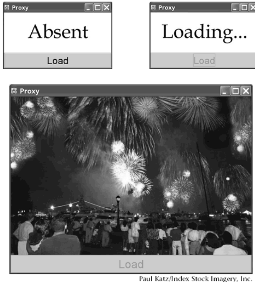
Figure 11.1. Three screen shots show a mini-application before, during, and after loading a large image. (Photo courtesy of Corbis, Inc.)
