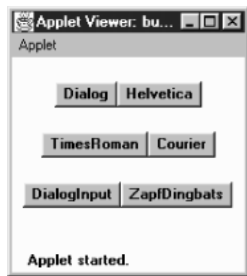
Figure 7.3: FlowLayout with hgap of 0 and vgap of 20
