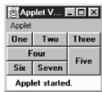
Figure 7.8: GridBagLayout with seven components on a 3x3 grid
