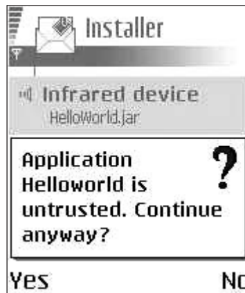
Figure 2.35 AMS checks that installation can continue.
