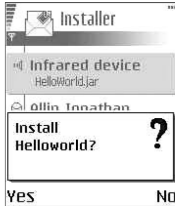
Figure 2.32 AMS checks that installation is required.
