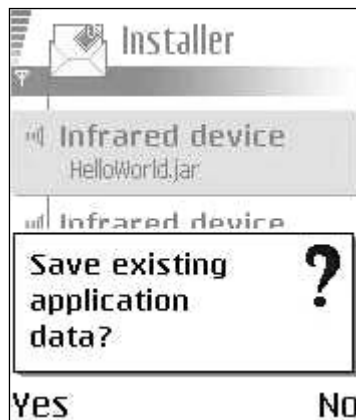
Figure 2.38 AMS checks whether to save existing data.
