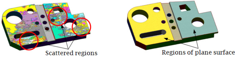
Fig. 4. Example of mesh segmentation, (a) an object segmented into many small regions due to a high sensitivity threshold, and (b) regions determined with a low sensitivity threshold
