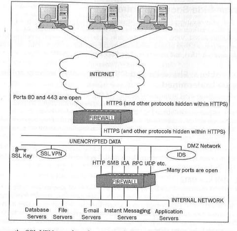
Because the SSL VPN tunnels various protocols through the external firewall and rebuilds them in the DMZ:
