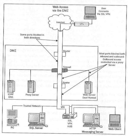
The traffic is routed into the DMZ, and then is terminated at the router. The IP address is now translated to a DMZ IP address, for example 10.10.10.10. The DMZ can then provide some authentication and allow the traffic to route to the trusted side of the DMZ. At this point the IP address can be translated to another IP address, like 192.168.10.12. The packets are then routed to the SSL VPN device (hub).
