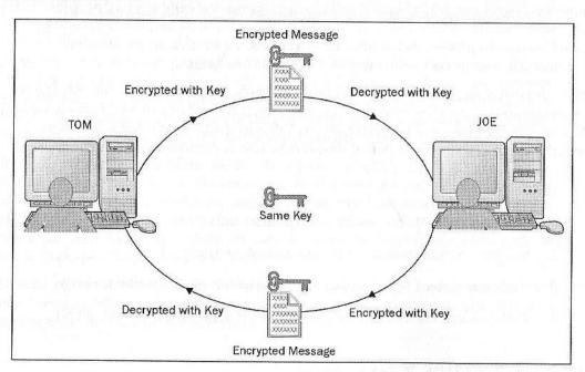
A **key** is a piece of data (usually a large number) that is fed to a cryptographic algorithm in order to encrypt plaintext into ciphertext or to decrypt ciphertext into plaintext. Utilizing the same algorithms with different keys will produce different results.
