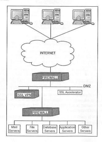
However, the use of an offloaded SSL accelerator can also impact architecture. For example, offloading SSL decryption from a less secure network to a more internal SSL processor can produce various effects. Examples of this scenario include:
