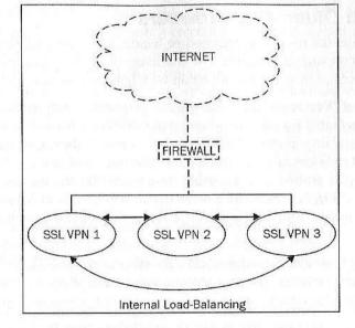
Even those SSL VPN products that lack an innate load-balancing capability can often be used in a load-balancing configuration through the addition of an external third-party load-balancing device placed in front of multiple SSL VPN appliances as shown below:
