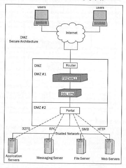
Legacy applications can be accessed though a set of portal connectors, also known as **portlets**. Some portlets provide legacy-based connectors, like a 3270 emulator connector.
