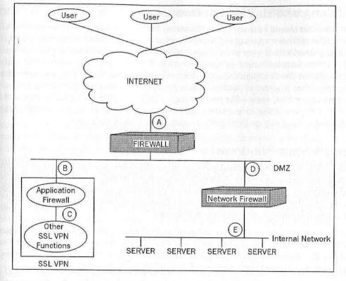
Filtering requests sent to the SSL VPN either as a function of the actual SSL VPN server or as a function of an application-level firewall situated in front of the SSL VPN can help address the problem of application-level vulnerabilities. Various types of filtering are discussed earlier in this chapter and, together, they can block rogue requests from crippling the SSL VPN, or from being able to reach and adversely affect internal systems.
