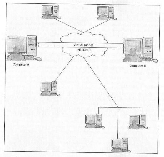
Tunneling is not a novel concept introduced with SSL VPN technology. It has been used in numerous technology implementations in the past, the most well known probably being **Internet Protocol Security** (**IPSec**) VPN (as described in chapter 1).
