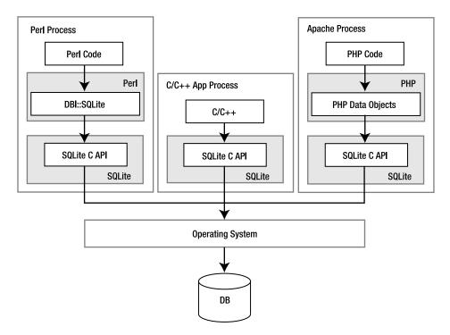
Figure 1-1. SQLite embedded in host processes
