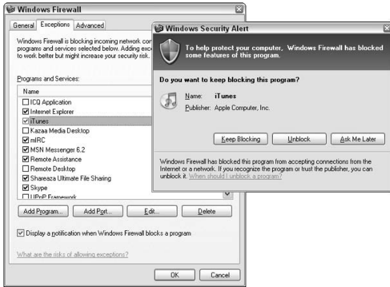
Figure 4-4: Clicking the Unblock button exempts a program so that it can bypass the firewall.
