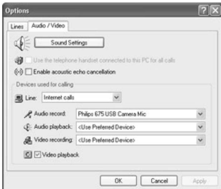
Figure 6-7: The Audio/Video page of Phone Dialer's Options dialog box lets you specify which devices to use for audio pickup and playback.
