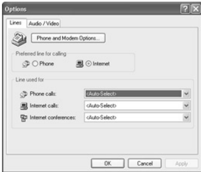
Figure 6-6: The Lines page of Phone Dialer's Options dialog box lets you specify your preferred line for different types of calls.
