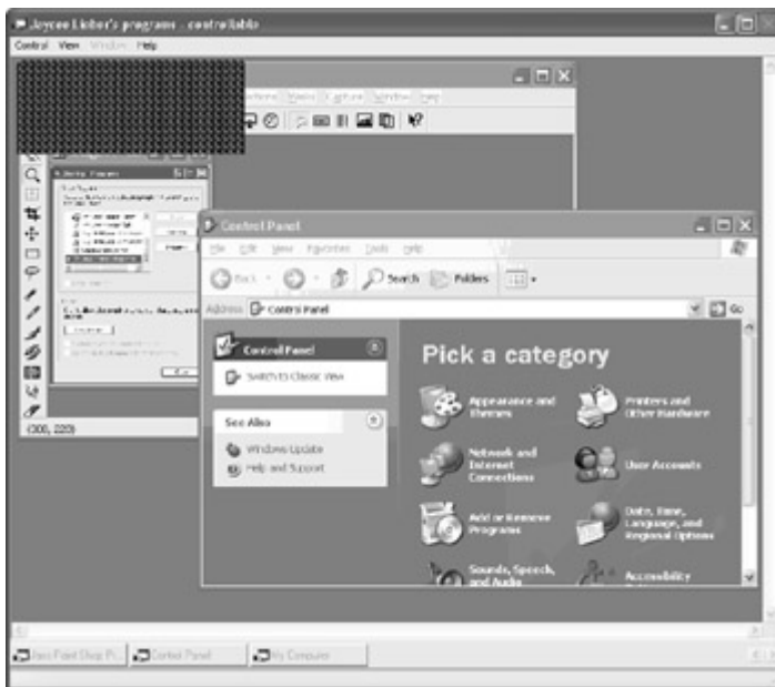
Figure 8-5: The shared programs appear in a Programs window like this on the other computer's screen. The Desktop appears blanked out if it's not being shared, and unshared programs can obscure the shared programs.
