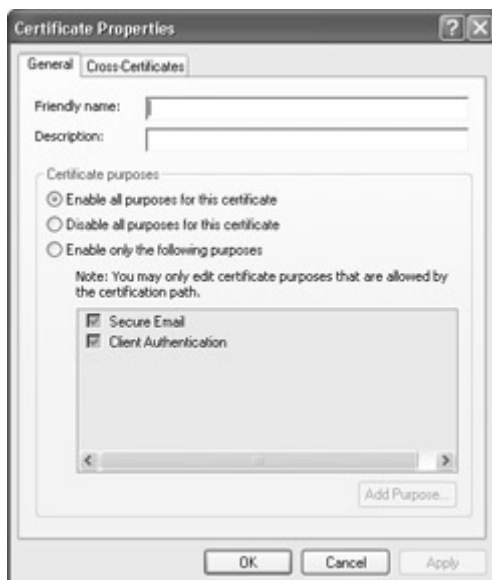
Figure 3-6: The General page of the Certificate Properties dialog box for a digital certificate lets you edit the friendly (descriptive) name and description for the certificate and specify the purposes for which you want to use the certificate.
