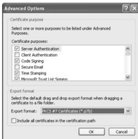
Figure 3-7: Choose a default format for certificates you export in the Export Format drop-down list in the Export Format group box in the Advanced Options dialog box.
