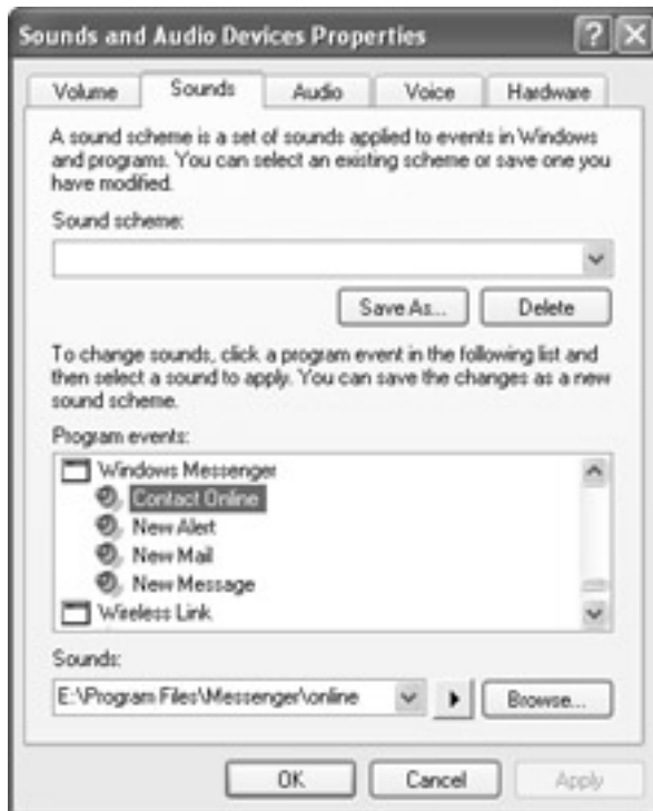
Figure 5-3: Use the Program Events list box on the Sounds page of the Sounds and Audio Devices Properties dialog box to specify different sounds for contacts, messages, and e-mail messages.
