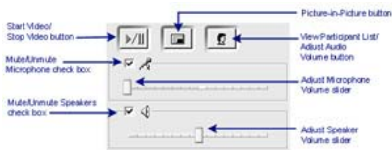
Figure 6-3: Display the audio controls to adjust the speaker volume or microphone volume.
