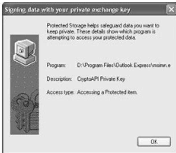
Figure 4-30: The second Signing Data with Your Private Exchange Key dialog box identifies the application that's requesting access to a protected item.
