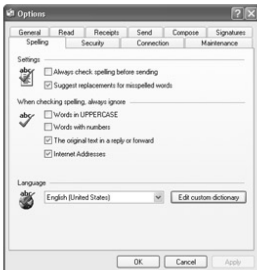
Figure 4-17: If you have Word or Office installed on your computer, you can choose spelling options on the Spelling page of the Options dialog box.
