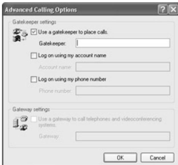
Figure 5-15: Use the Advanced Calling Options dialog box to specify any gatekeeper or gateway computer through which your computer connects to the network.
