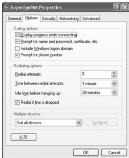
Figure 2-4: Choose dialing and redialing options on the Options page of the Properties dialog box for the Internet connection.
