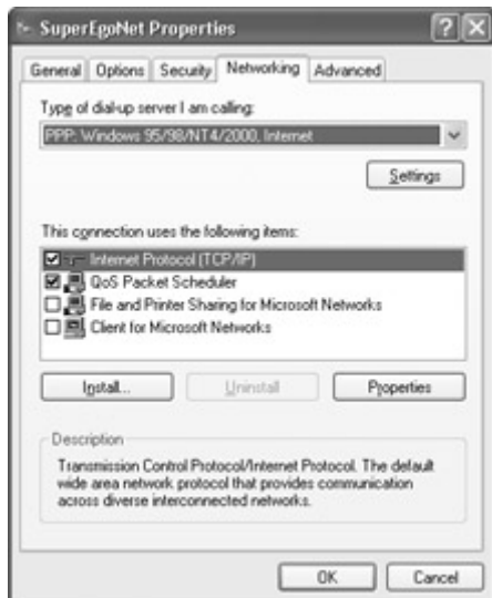
Figure 2-7: In most cases, the Network Setup Wizard chooses appropriate options on the Networking page of the Properties dialog box for a connection.
