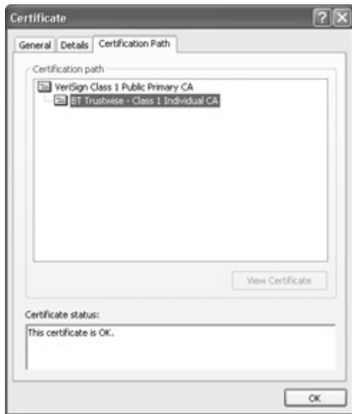
Figure 3-5: The Certification Path page lets you examine the certification path from the certification authority to the holder of the certificate.
