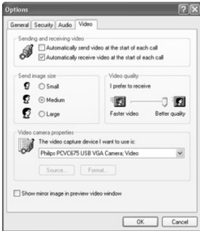
Figure 5-18: The Video page of the Options dialog box lets you specify the size and quality of video you send and receive.
