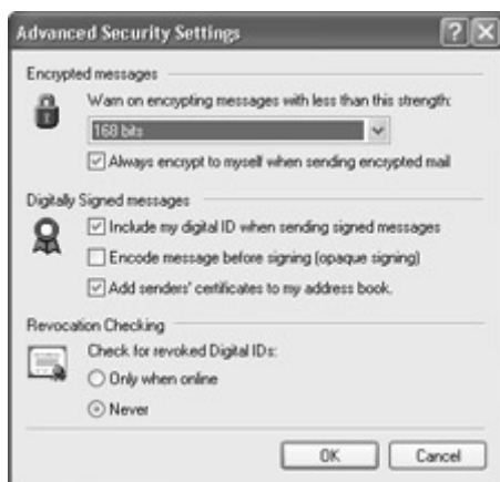
Figure 4-16: If you're encrypting or digitally signing messages, check that the options in the Advanced Security Settings dialog box have suitable settings.
