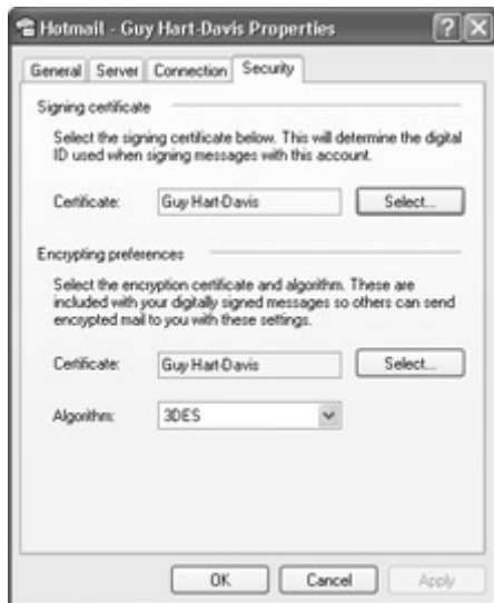
Figure 4-25: On the Security page of the Properties dialog box for a connection, specify the certificates for digitally signing messages and encrypting messages and attachments.
