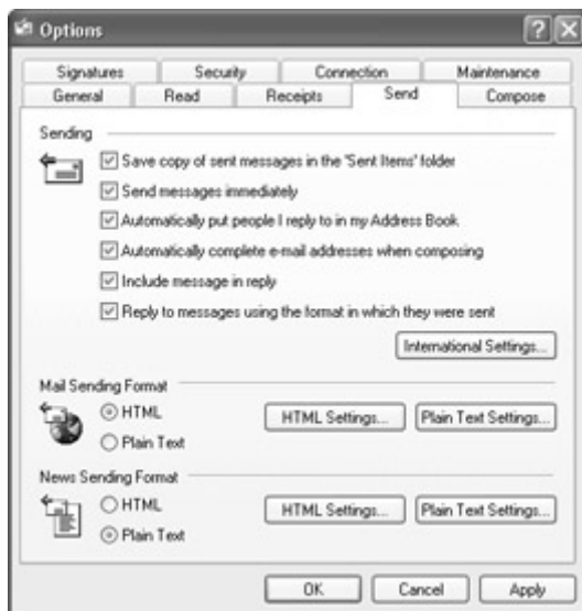
Figure 4-11: The Send Messages Immediately check box on the Send page of the Options dialog box controls whether Outlook Express sends messages immediately or queues them when you issue a Send command.
