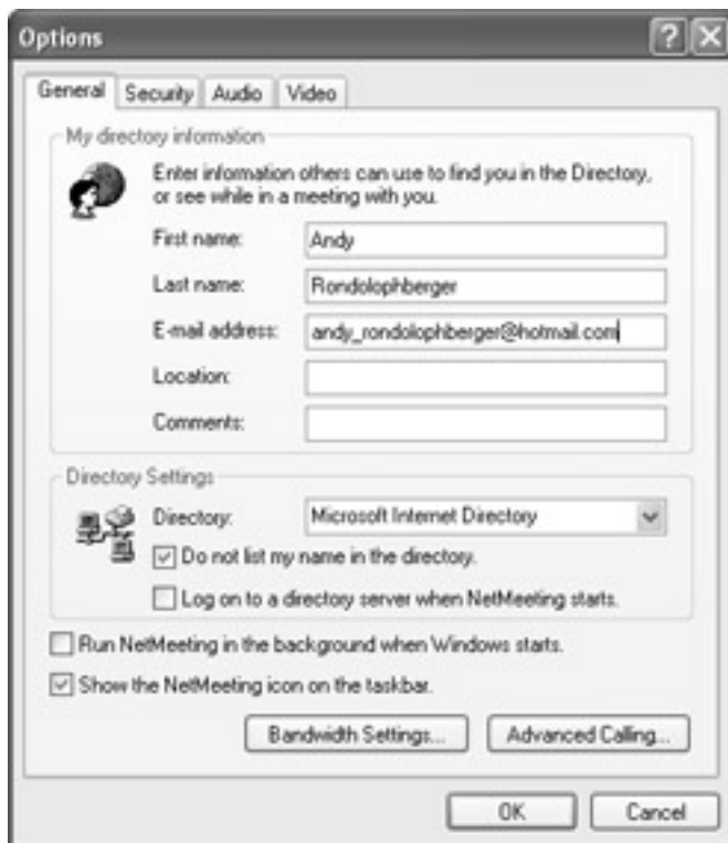
Figure 5-14: The General page of the Options dialog box for NetMeeting contains options for specifying your directory information, choosing whether to log into a directory, and specifying whether to run NetMeeting when Windows starts.
