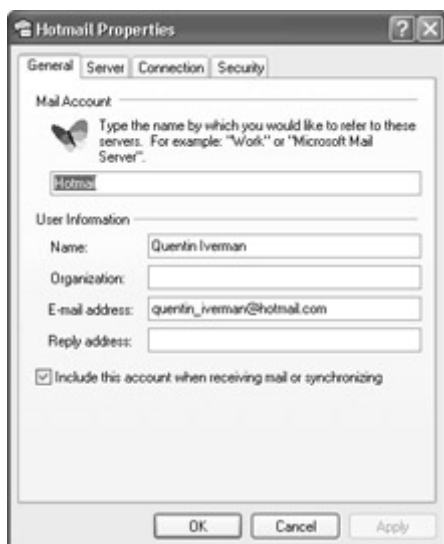
Figure 4-21: The General page of the Properties dialog box for an e-mail account lets you change the account's name, your name and organization, your e-mail address and reply address, and whether to check the account when sending and receiving mail.
