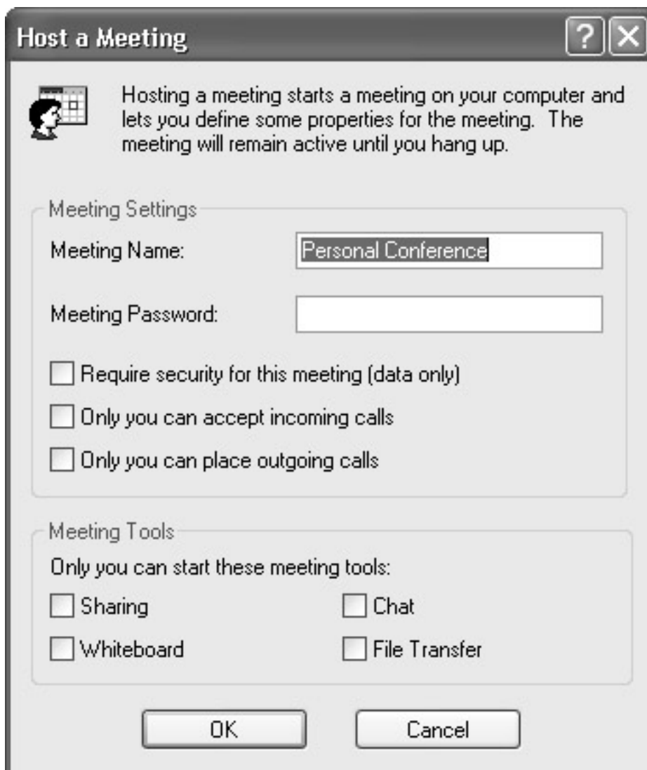
Figure 5-23: The Host a Meeting dialog box lets you set a password, security restrictions, and tool restrictions for the meeting.
