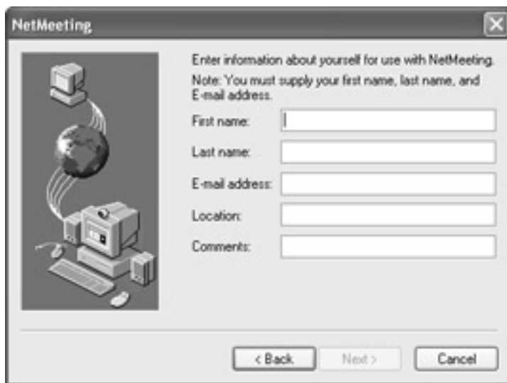
Figure 5-12: On this page of the NetMeeting setup routine, enter the first name, last name, and e-mail address that you want NetMeeting to display for you.
