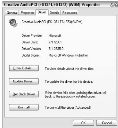
Figure 10-4: Use the Update Driver button to replace your PC's sound device software.
