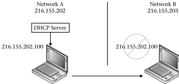
**Figure 20-16** DHCP network with moved workstation
