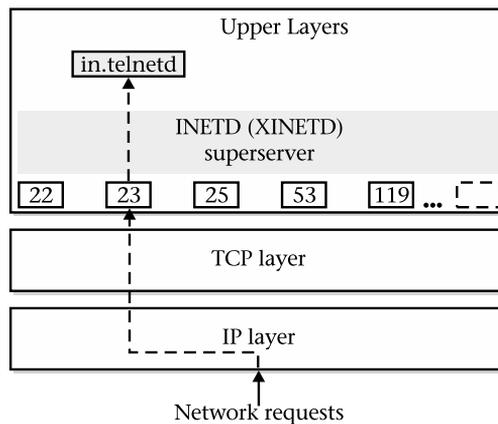
**Figure 10-4** `inetd` operation with a Telnet request
