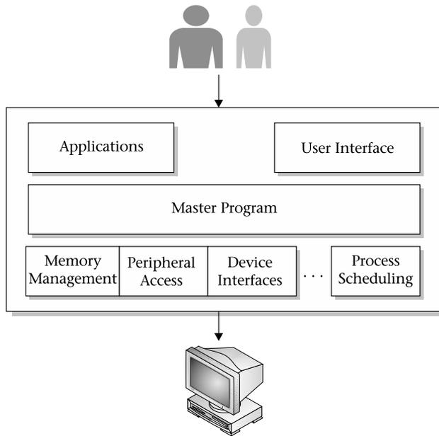
**Figure 1-2** Diagram of a typical operating system
