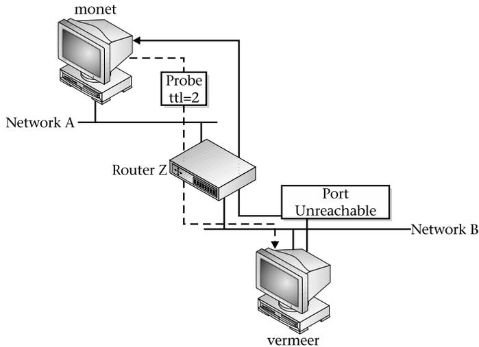
**Figure 12-3** Using traceroute with two hops in network
