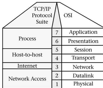
**Figure 10-1** TCP/IP and the OSI networking model
