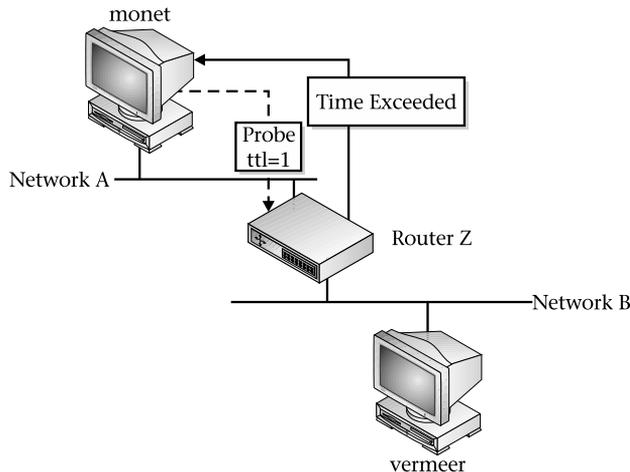
**Figure 12-2** Using `tracert` with single hop in network
