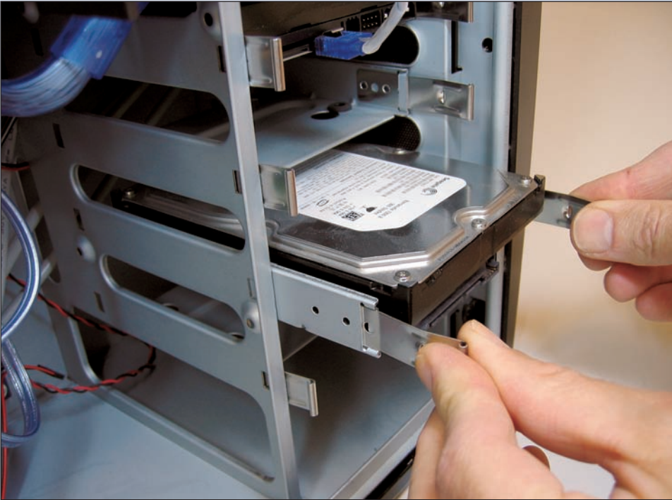
Color Plate 26: Some cases come with rails to screw onto the drives, making them easy to slide in and out of their drive bays.
