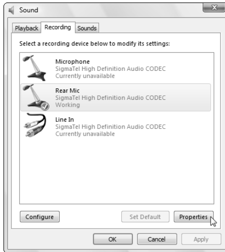
Figure 11-6: Click your microphone's listing and click the Properties button to set its recording levels.
