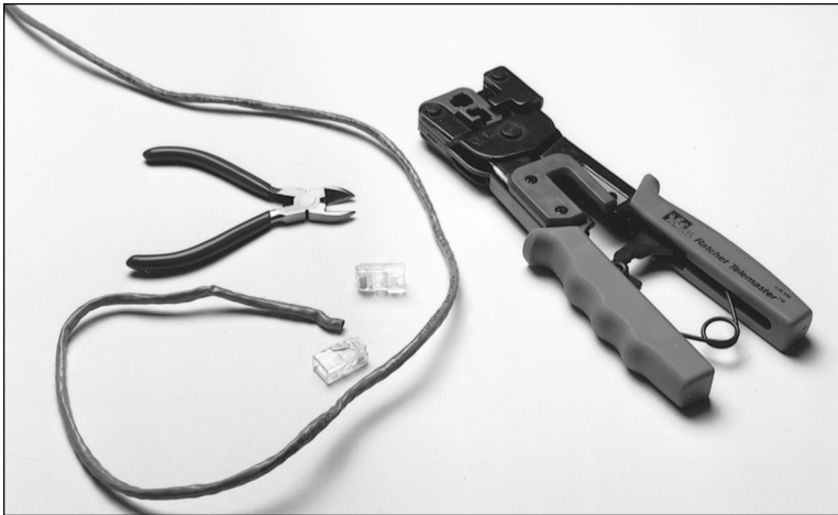
Figure 20.17 You'll need wire strippers, a crimping tool, bulk UTP cable, and RJ-45 connectors to make your own 10BASE-T (100BASE-T) cables.
