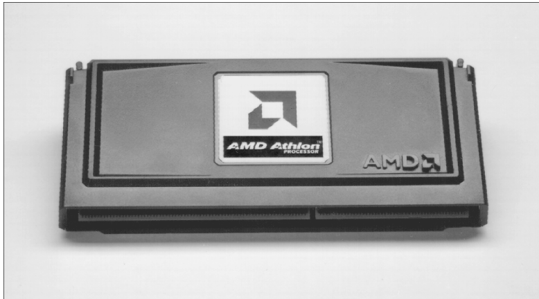
Figure 3.57 AMD Athlon processor for Slot A (cartridge form factor).
