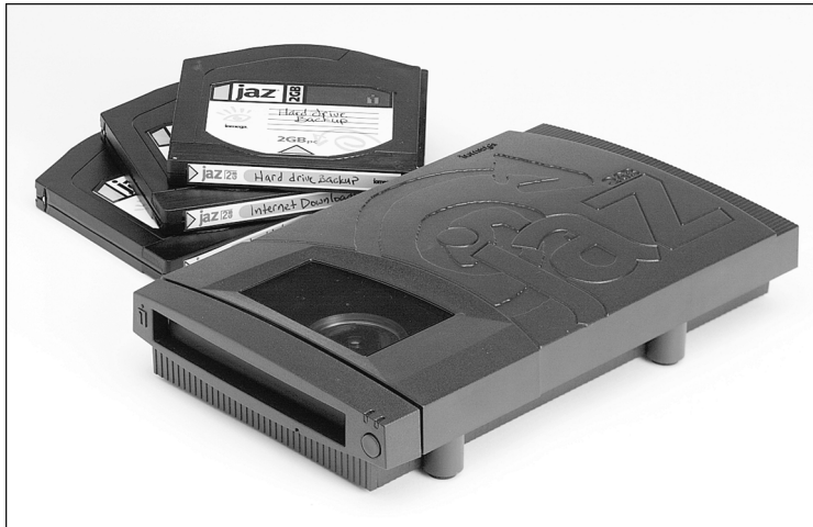
Figure 12.4 A 2GB external Jaz drive and media. Photo courtesy of Iomega Corporation.
