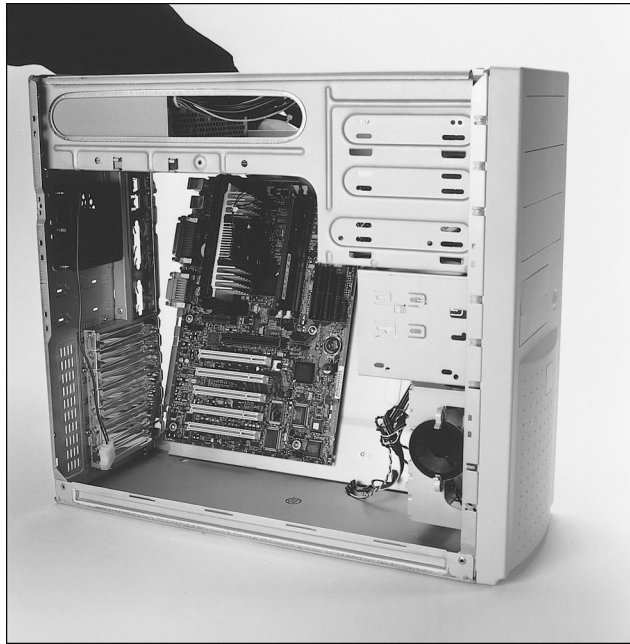
Figure 22.16 Installing the motherboard and tray into the chassis. Case courtesy of PC Power & Cooling, Inc. Motherboard courtesy of Intel Corporation.
