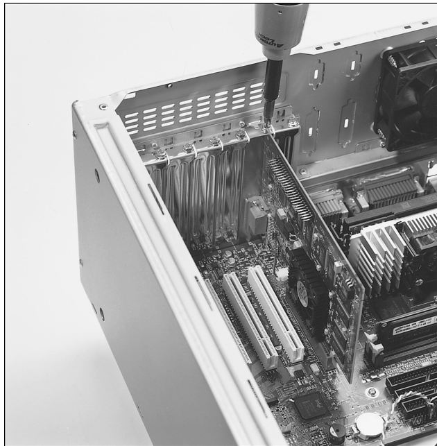
Figure 22.29 Installing the screw to retain the card. Motherboard courtesy of Intel Corporation.
