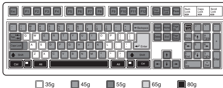
Figure 18.6 Force levels used on Key Tronic keyboards with Ergo Technology.
