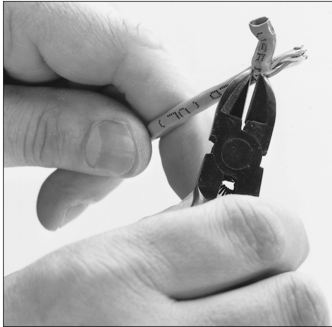
Figure 20.18 Carefully strip the cable jacket away to expose the four wire pairs.
