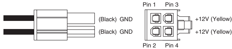
Figure 21.15 An ATX12V power connector.
