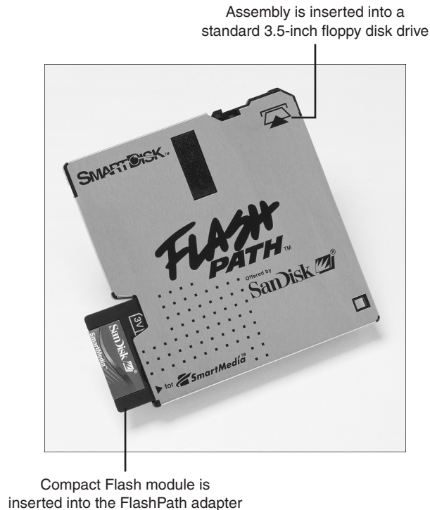
Figure 12.10 A CompactFlash module is inserted into the FlashPath adapter; the assembly is then inserted into a standard 3 1/2" floppy drive. Photo courtesy of SanDisk.
