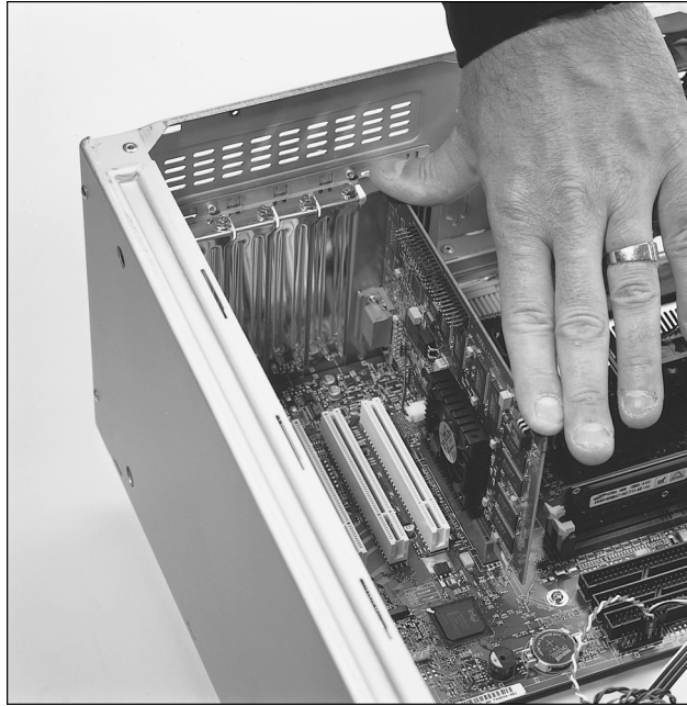
Figure 22.28 This photo shows a video adapter being inserted into the slot. Motherboard courtesy of Intel Corporation.
