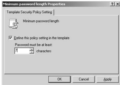
FIGURE 1.5 The individual policy setting dialog box for setting a minimum password length
