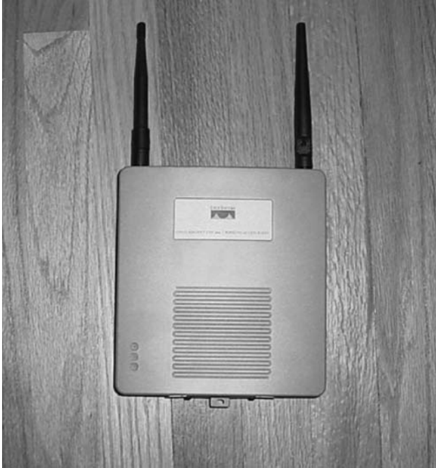
Figure 10.14 Cisco 1200 access point detail.
