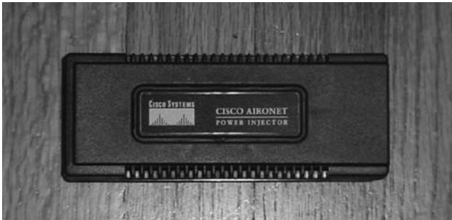
Figure 10.11 Cisco power injector detail.
