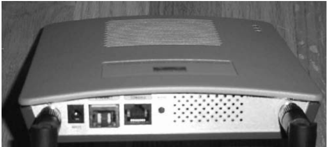
Figure 10.16 Cisco 1200 side port detail.
