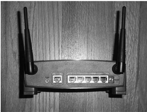
Figure 10.4 Older-style Linksys access point side port detail.
