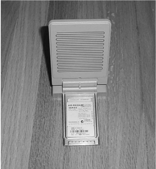
Figure 10.15 Cisco 1200 removable 802.11a radio detail.
