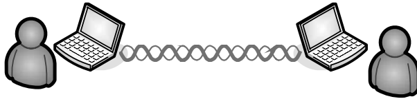
Figure 6.1 Ad Hoc or Independent Basic Service Set (IBSS) diagram.
