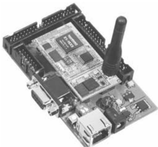
Figure 10-2: The Micro BlueTarget Starter Kit uses a standard Micro BlueTarget and adds RS-232 and Ethernet ports, which is ideal for developers who need to create quick prototypes and proofs of
