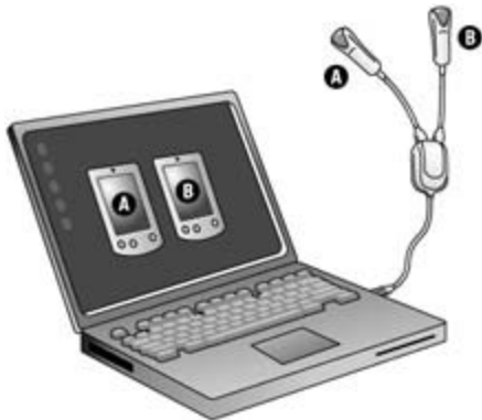
Figure C-1: With the TDK Bluetooth Developer's Kit and the PalmOS emulator, you can develop, deploy, and test your Java Bluetooth applications all within the environment of your development machine.
