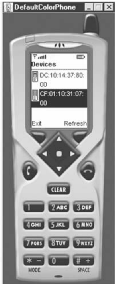
Figure 5-4: After a remote device is found, we now go into stealth mode (i.e., nondiscoverable).
