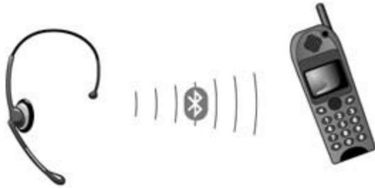
Figure 2-4: You can only connect to one Bluetooth device at a time if you have hardware that only supports point-to-point communication.
