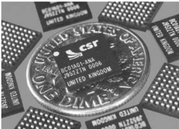
Figure 2-2: The CSR BlueCore 1. This single-chip solution includes a microprocessor, RAM, I/O controller, and Bluetooth implementation in a single package! This is most likely the smallest radio that you've ever seen.
