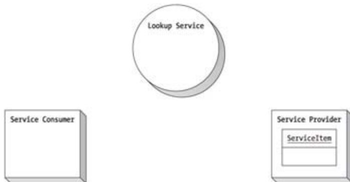
Figure 12-1: These three entities must exist before a Jini federation is established. The federation itself hasn't been formed because the entities don't know anything about each other yet.
