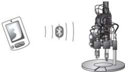
Figure 10-4: A Bluetooth PDA receiving the status from a fixed-wireless commercial system— a Bluetooth-enabled machine in a manufacturing facility
