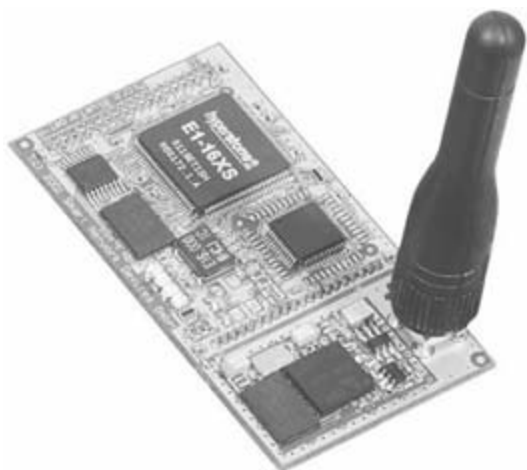
Figure 10-1: The Micro BlueTarget standard version is a small form factor embedded system with a board outline of just 3.25.9 cm! This is a great solution for OEMs that want to make their devices Bluetooth enabled.
