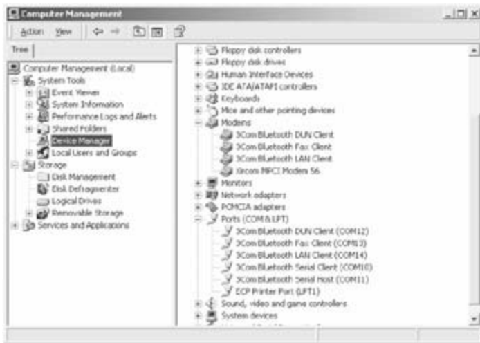
Figure 2-8: As you can see in Windows 2000, the operating system thinks that COMM10 and COMM11 are actual serial ports!
