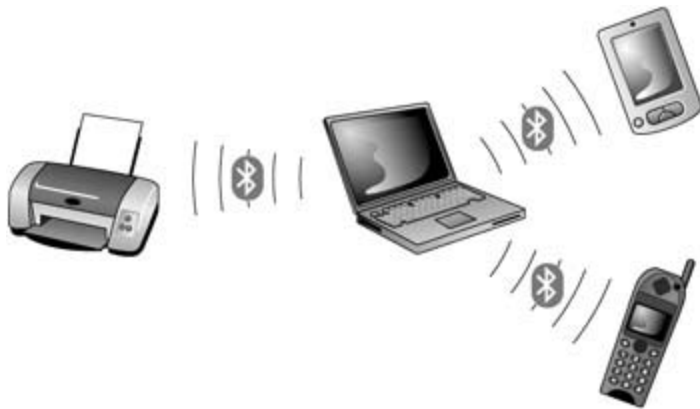
Figure 2-5: You can connect to up to seven Bluetooth devices at a time if you have multipoint-capable hardware.
