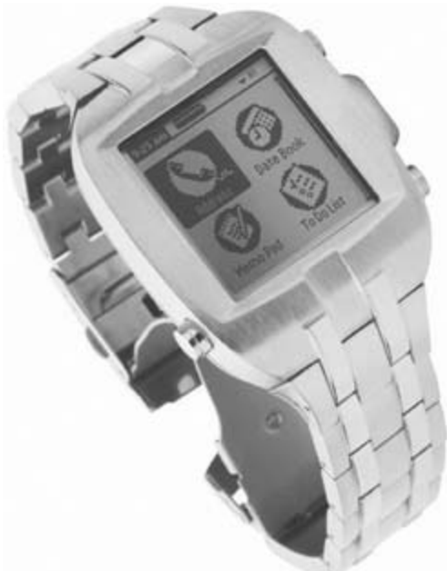
Figure 1-3: Although the Fossil Wrist PDA doesn't contain any Bluetooth hardware, it does come preloaded with a Bluetooth-enabled OS—the Palm OS 4.1. Palm OS is a registered trademark of Palm, Inc.
