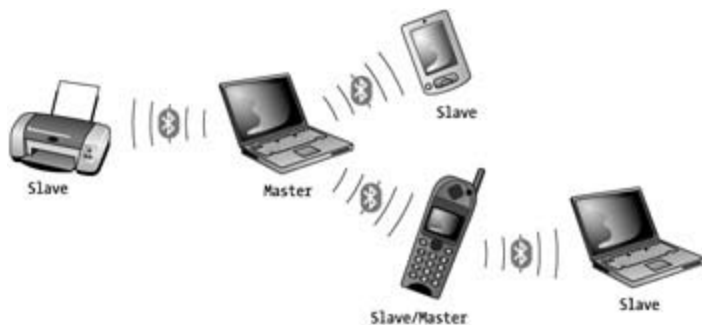
Figure 2.11: A scatternet is formed when a slave in one piconet is the master in another piconet.
