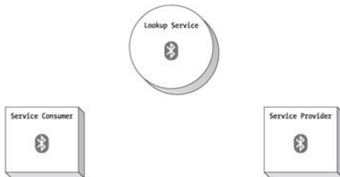
Figure 12-8: In an all-Bluetooth Jini federation, all the devices participating in the federation must be Bluetooth enabled. This federation is wireless.
