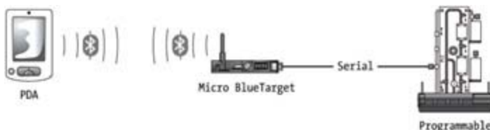
Figure 10-10: Using the Micro BlueTarget to create a fixed-wireless system
