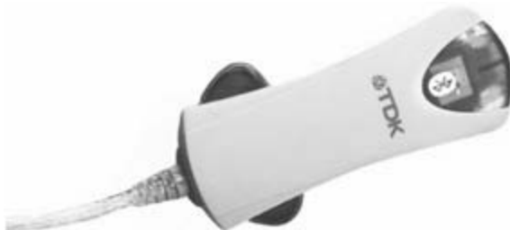
Figure 5-5: The TDK USB Bluetooth device using a CSR Bluetooth radio
