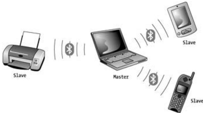
Figure 2-10: In a piconet, the slaves can only communicate to the master.
