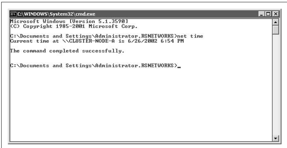
Figure 3-6. Viewing the Net Time command in the command prompt
