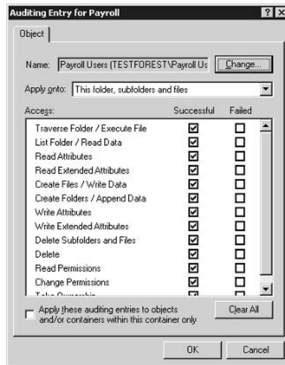
FIGURE 11.6 Auditing the Payroll Users security group for successful access to the folder
