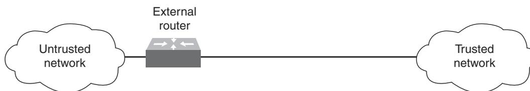
**Figure 3.7** A Packet-Filtering Router.
