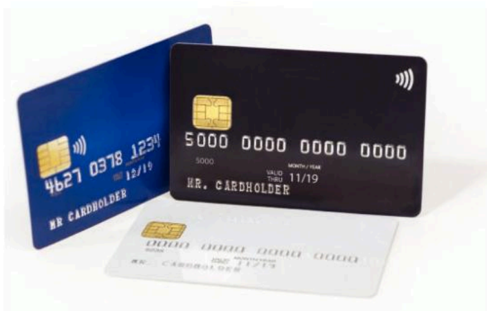
Fig 1.7 Smart cards have a built-in electronic circuit and a set of gold-coloured contacts
