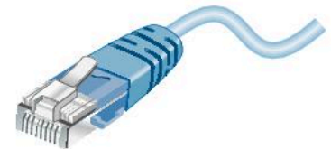
Fig 3.7 Ethernet cables are used as network cables
