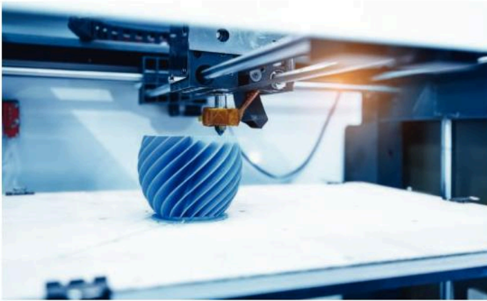
Fig 1.11 3D printers create a model layer by layer
