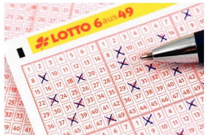
Fig 1.8 Data can be entered into a computer in different ways. Lottery slips are an example of optical mark recognition (OMR)
