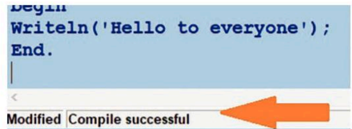
Fig 11.4 Compiling the program shows a message at the bottom of the screen that there were no syntax errors
