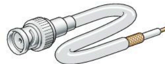
Fig 3.8 Coaxial cable is used for televisions, video and cable TV
