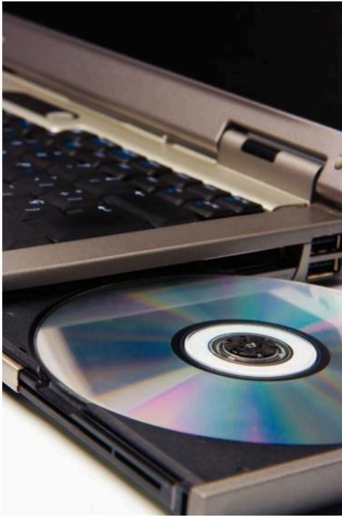
Fig 1.20 Optical disks can store large amounts of data and typically used for storing digital data, movies and gaming software
