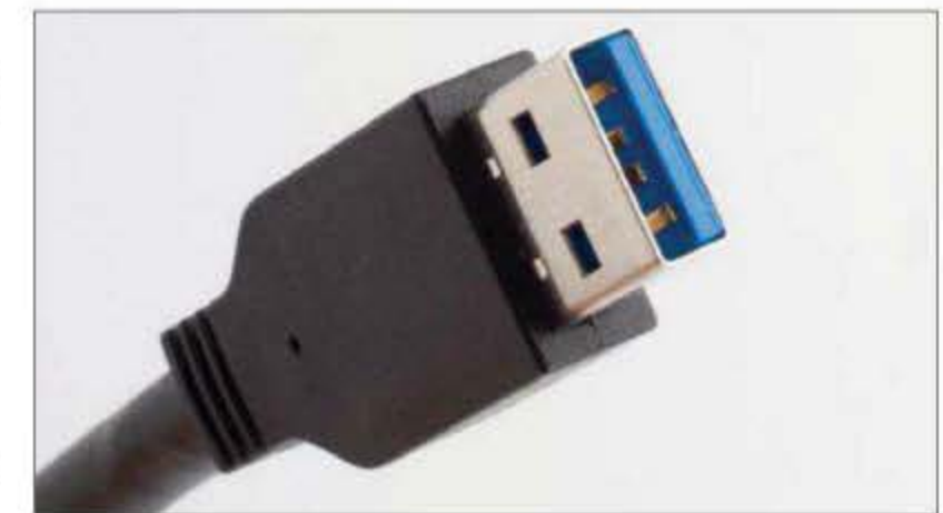
↑ USB 3.0 connectors look and act in the same way as their USB 2.0 predecessors. But the internal spec means connectivity speeds are quicker
