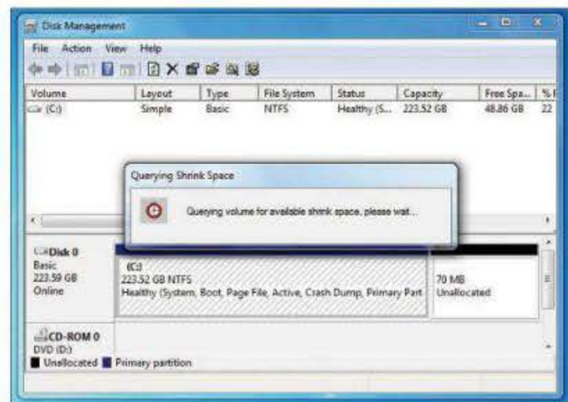
1 First, check how much space you can use for your partition. Go to Control Panel, Disk Management and right-click on the drive you want to partition. Windows will determine how much unallocated space is available. You'll use this to create a new, 'Simple' drive.
