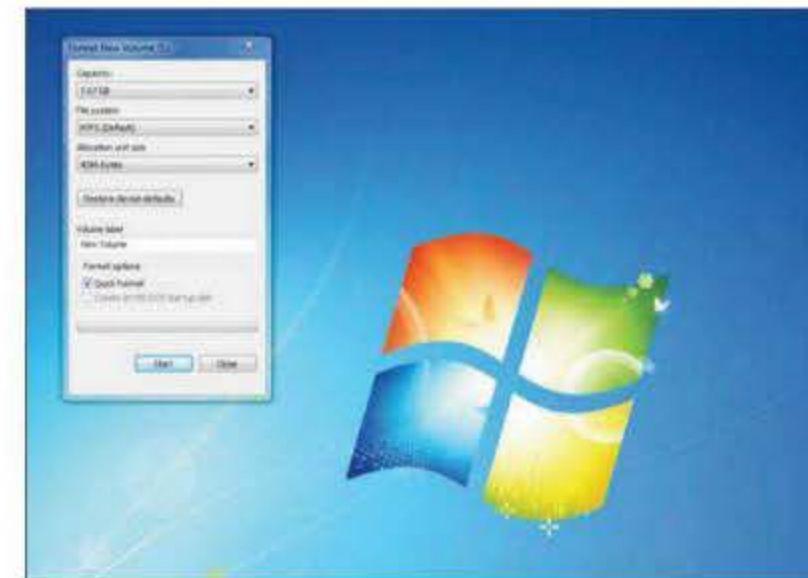
3 Right-click within the unallocated disk space pane in the Virtual Disk utility and select 'Create new Simple drive'. You can choose between FAT and NTFS drive types. Stick with the latter and click to proceed. Either accept the default drive name such as E or type in your own. Allow Windows to perform a quick format of the existing content.
