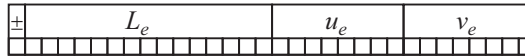
Figure 6.8 Storage arrangement for a pixel in 32 bit LogLuv format. (After images courtesy of Greg Ward.)
