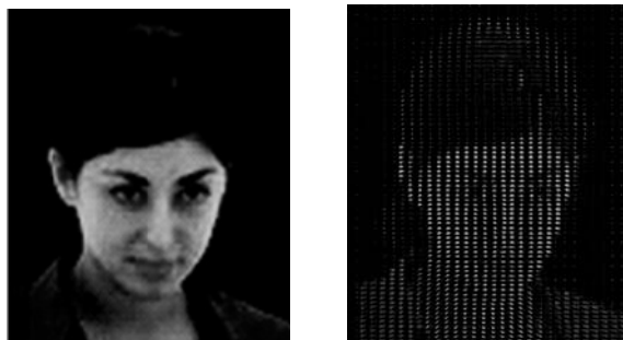
Figure 8.27 All the reflectance function images captured from the light stage spotlights can be tiled into a single texture image (right). A captured image is shown on the left. (Courtesy of Paul Debevec.) (See Color Plate X.)
