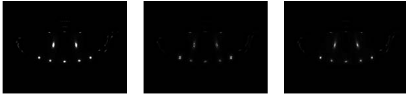
Figure 8.20 Differences between the BRDFs in the linear span of the PCA basis vectors and the Gaussian basis representation. A measured BRDF is shown at the left. In the center is an implausible BRDF from a nearby “point” in the linear span. The right image is a BRDF at a comparably close point in the Gaussian subspace; the BRDF is different, but still physically plausible. (From [Matusik et al. 03] © 2003 ACM, Inc. Included here by permission.)
