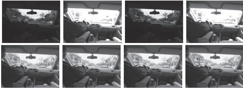
Figure 6.12 High dynamic range video of a driving scene. Top row: input video with alternating short and long exposures. Bottom row: high dynamic range video (tone-mapped). (From [Kang et al. 03] © 2003 ACM, Inc. Included here by permission.) (See Color Plate IX.)
