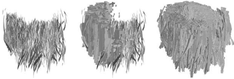
Figure 8.70 Hair “ribbons” in a 3D volume of detected hair fibers. The left image is from a single viewpoint; the middle image is from two viewpoints; the right image comes from 24 viewpoints. (From [Jakob et al. 09] © 2009 ACM, Inc. Included here by permission.)
