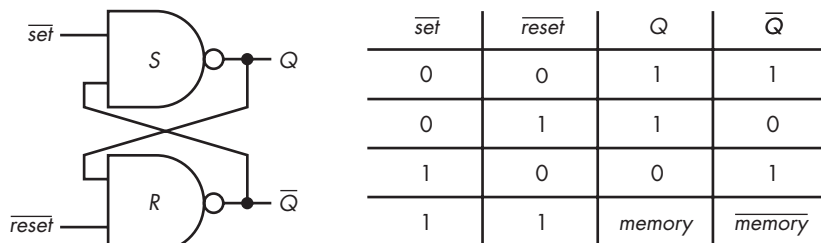
Figure 3-5: An S-R latch
