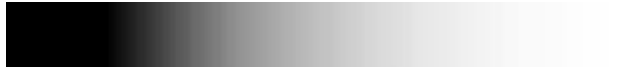
Figure 7. A typical lightness scale, with black at one end and the brightest possible white at the other.
