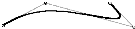
Figure 5. Spline function estimated from four control points. The gray lines denote the control polygons connecting the control points.
