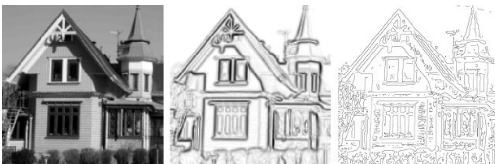
Figure 3. Edge detection: (left) A gray-level image of size 180 \times 180 pixels, (middle) The negative value of the gradient magnitude |\nabla L| computed at t = 1 . (right) Differential geometric edges at t = 1 with a complementary low threshold \sqrt{t}|\nabla L| \geq 1 on the gradient magnitude.
