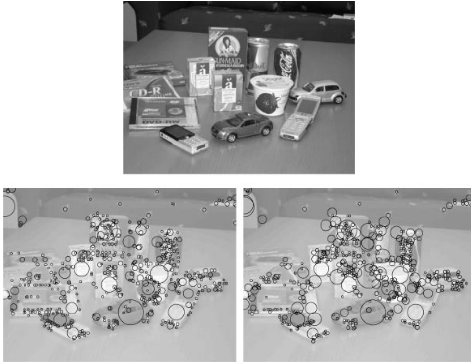
Figure 8. Scale-invariant feature detection: (top) Original gray-level image, (bottom left) The 1000 strongest scale-space extrema of the scale normalized Laplacian \nabla_{norm}^2 . (bottom right) The 1000 strongest scale-space extrema of the scale normalized determinant of the Hessian \det \mathcal{H}_{norm} L . Each feature is displayed by a circle with its size proportional to the detection scale. In addition, the color of the circle indicates the type of image feature: red for dark features, blue for bright features, and green for saddle-like features.
