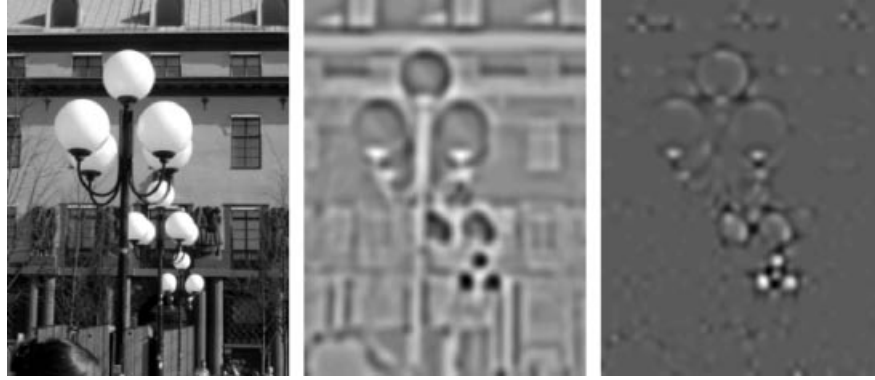
Figure 4. Differential descriptors for blob detection / interest point detection: (left) A gray level image of size 210 \times 280 pixels, (middle) The Laplacian \nabla^2 L computed at t = 16 . (right) The determinant of the Hessian \det \mathcal{H}L computed at t = 16 .
