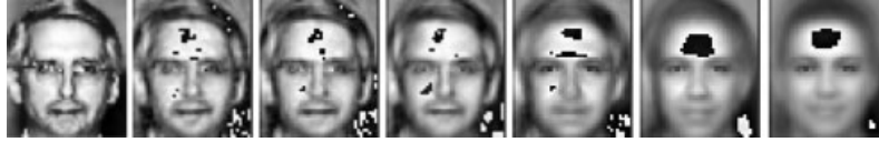
Figure 5. Original image [size 48 \times 42 (i.e., 2016)] and the reconstructed image using 300, 200, 100, 50, 20, and 10 leading components, respectively (32).
