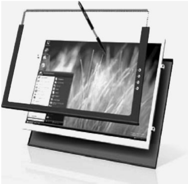
Figure 1. A digitizing tablet shown in the configuration where the digitizer is mounted on top of the screen (2) .
