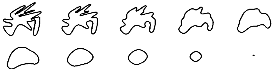
Figure 2. A contour moving with the curvature flow in the level set framework. Note the fast evolution in the regions where the contour bends more than the other regions.
