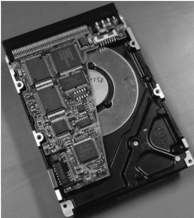
Figure 1. Typical components of an HDD: (a) view of inside parts of the HDD and (b) view of the printed-circuit-board side.
