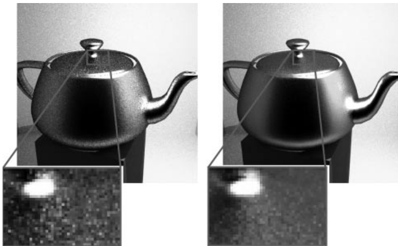
Figure 7. Importance can substantially reduce the noise level in the image. Both the left and right images were computed with MC ray tracing using 100 samples per pixel. Uniform hemisphere sampling was used for the image on the left; importance sampling was used for the image on the right.
