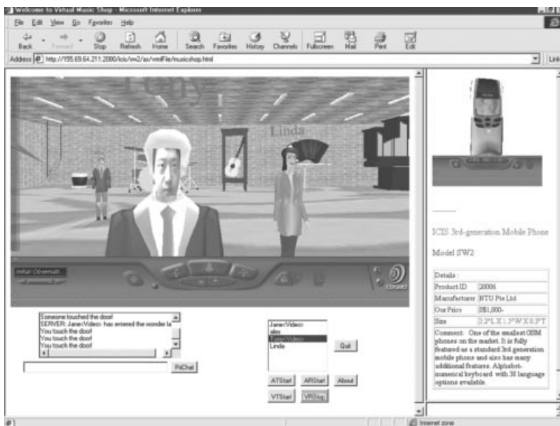
Figure 4. Web-based 3-D VRML virtual community CVE with live audio and video avatar face. (Note: Live audio and video data are transmitted in peer-to-peer.)
