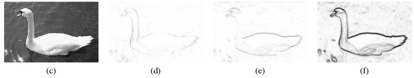
Figure 1. The convolution mask to detect (a) the vertical edges and (b) the horizontal edges, (c) An input image. Resulting (d) vertical edges after convolving (a) with (c), and (e) horizontal edges after convolving (b) with (c). (f) The gradient magnitude image generated using (d) and (e) for highlighting the boundary of the object.
