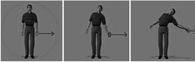
Figure 3. Changing the posture of a human figure by using inverse kinematics. The user specifies the motion of the hand, and the system calculates the joint angles of the body automatically.
