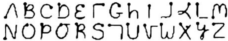
Figure 3. The Graffiti character set developed by palm computing. The dot on each character shows its starting point.
