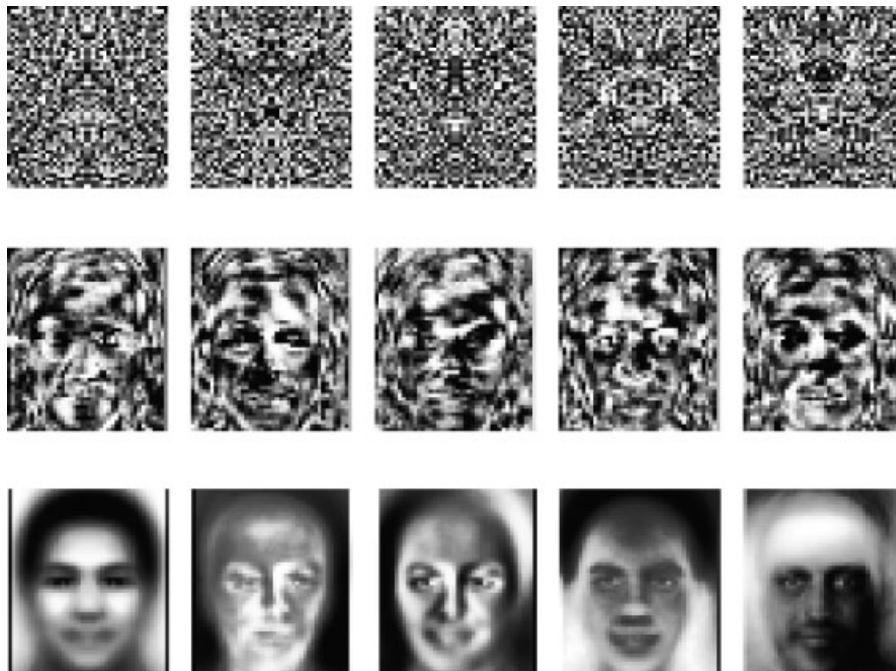
Figure 8. Different projection bases constructed from a set of 444 individuals, where the set is augmented via adding noise and mirroring. (Improved reconstruction for facial images outside the training set using an extended training set that adds mirror-imaged faces was suggested in Ref. 14.) The first row shows the first five pure LDA basis images W , the second row shows the first five subspace LDA basis images W\Phi , the average face and first four eigenfaces \Phi are shown on the third row (18).
