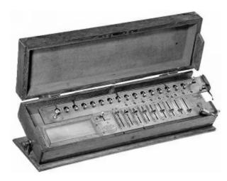
1820: Charles Xavier Thomas invents the arithmometer (first digital mechanical calculator to be used on a wide scale).
