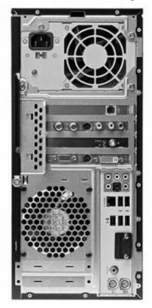
You can see the power supply at the top of the picture; it has a place to plug in the power cord (on the left), and a vent to allow air flow (on the right).
