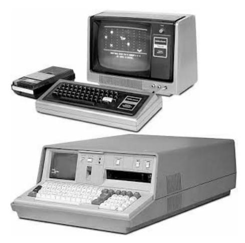
These original PCs had basic functions and components, including: memory, keyboard, card reader, card recorder (data could be stored from the computer on magnetic tape or magnetic card) and processor.
