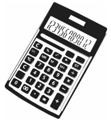
In the above picture, the liquid crystals are the "|" marks that block the light from coming through and thereby display the numbers. For example: the number 2 contains 5 liquid crystals:
