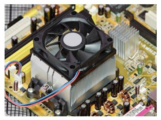
In this picture, the fan is mounted on top of a heat sink on a printed circuit board. You can also see a computer fan on the top right of the tower pictured earlier in this chapter. Sometimes you can hear a whirring sound inside your computer; that's the fan blades spinning.
