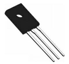
This is actually pretty large as computer parts go – it is about half an inch long. Computers nowadays use much smaller parts to perform the same function of storing a binary digit (a bit). We are using an older, larger device just to help illustrate the way this works. You would need a microscope to see the current devices in real life.
