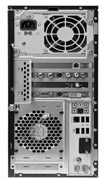
These connection points that you plug into are called "ports." Most attach directly into the motherboard, as you can see here:
