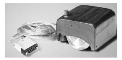
A mouse is a device that allows the user to interact with the visual display screen of the computer. It is a movable device about the size of a small hand.
