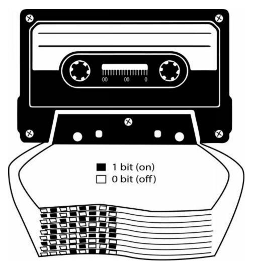
The black squares represent areas on the tape where a particular quality of magnetic energy was stored by stacks of magnets. The marks left by these magnets can be read by machines using heads (machine parts that pick up [read] and transfer electronic signals). They operate in the same, basic fashion as punched cards and tape.
