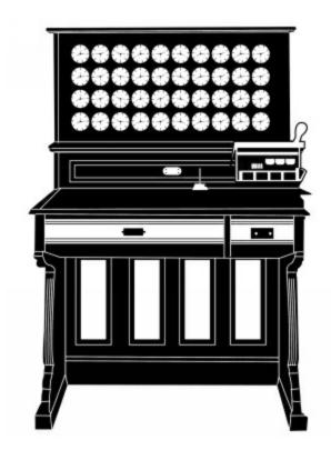
the tabulating machine (machine run off electricity and used punch cards to calculate the U.S. census [population count]).
