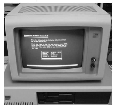
With a black and green monochrome screen, for example, each spot on the screen has two possible states: on (green) or off (black).
