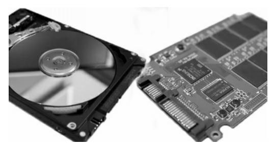
The drive on the left contains disks, and the drive on the right is composed of chips and transistors.
