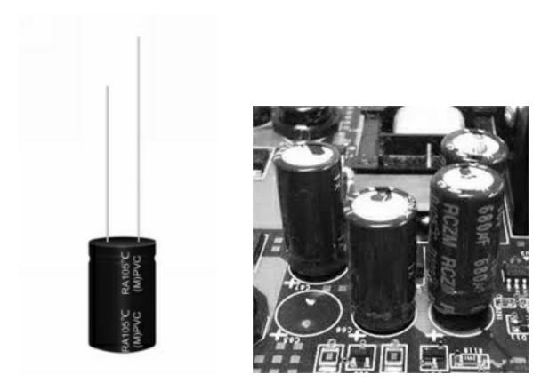
Some look like little batteries plugged into boards (thin, flat boards that contain complex electronic circuits). With some devices (like routers) you need to wait a few seconds after turning it off to ensure all the electricity is drained from the capacitors to make sure it is indeed off. Meaning, if you just click off and on, the device may not actually be fully off – give it a minute.
