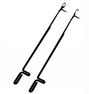
The needles were mounted at the top of the loom. There was one needle for each warp thread in the fabric you were making. Each needle could be set (using a lever, which is a handle used to operate part of a machine) to either lift a warp thread or not lift it.
