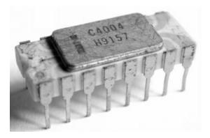
1971: Intel releases the first CPU (central processing unit) – the Intel 4004.
