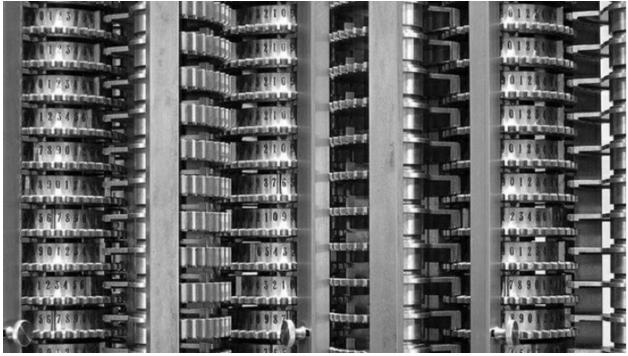
The machine also had a central set of gears which supervised and controlled the rest of the mechanism. This main set of gears could be considered the machine's "central processing unit" – they controlled all of the other gears in the machine. We will describe a modern central processing unit in further detail later in this book, but simply put, it is the main part of the computer that performs calculations and controls the various parts of the computer.
