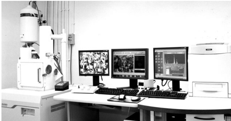
Fig. 4.23 The JEOL 6490 scanning electron microscope. This microscope has a resolution of 3 nm at an electron beam energy of 30,000 V. The sample chamber is differentially pumped which allows for pressures of up to 50 Pa (0.4 Torr) at the sample chamber while maintaining a high vacuum for the electron optics. This permits imaging in a humid atmosphere, maintaining the state of biological samples and avoiding electron beam charging for insulating samples. (Courtesy of JEOL USA Marketing.)
