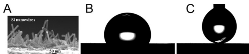
Fig. 9.25 (a) Structure of the surface on which a dense array of Si nanowires have been grown. (b) A water drop on a plane surface and (c) a water drop on a nanotextured surface. (From Rosario et al. 36 , J. Chem. Phys. 2004, with permission from the American Chemical Society.)
