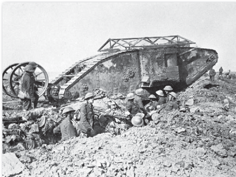
British Mark I tank with antibomb roof and "tail," 1916. Courtesy of the Imperial War Museum, London; photographs, Camera Press
