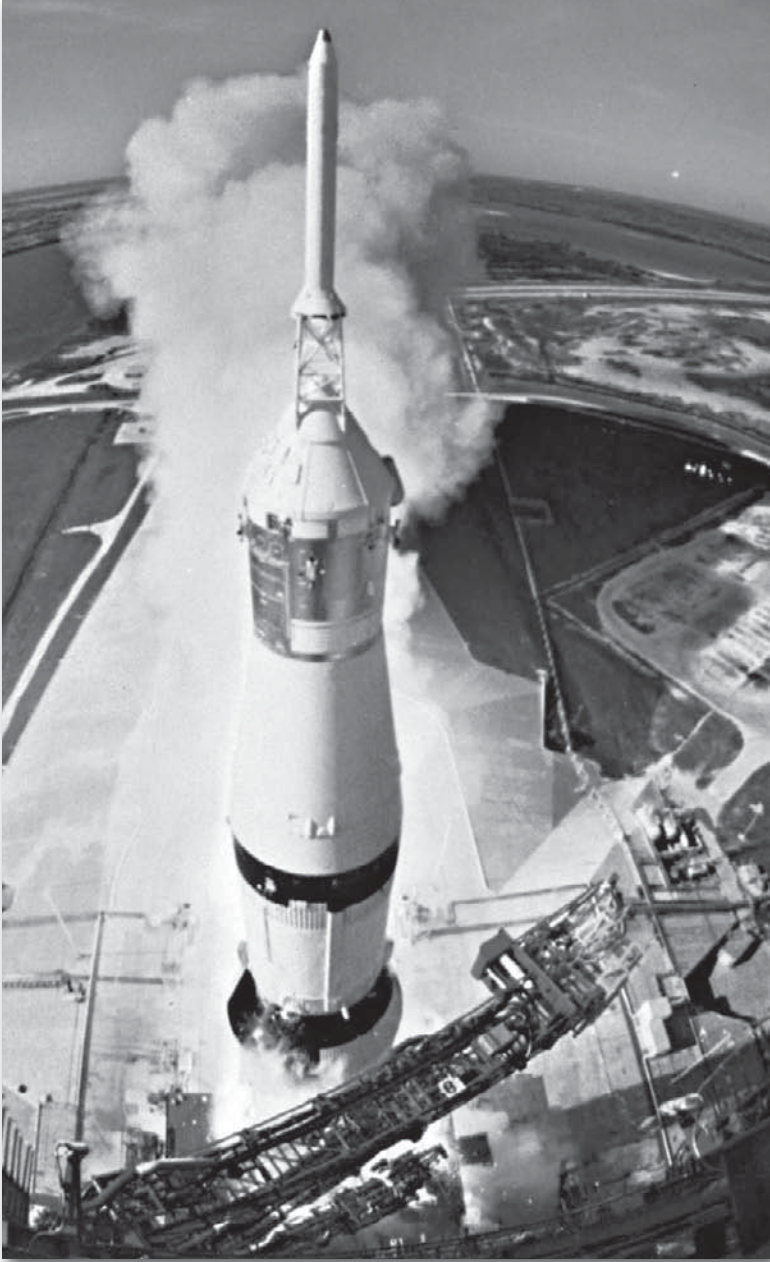
The Apollo 15 spacecraft lifts off from Cape Kennedy, Florida, U.S., atop a Saturn V three-stage rocket, July 26, 1971. A camera mounted at the mobile launch tower's 360-foot (110-m) level recorded this photograph. NASA
