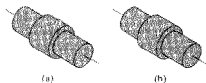
Figure 15.1 Two parts of identical shape and size but different manufacturing requirements: (a) 1,000,000 pc/yr, tolerance = \pm 0.010 in, material = 1015 CR steel, nickel plate; and (b) 100 pc/yr, tolerance = \pm 0.001 in, material = 18 - 8 stainless steel.
