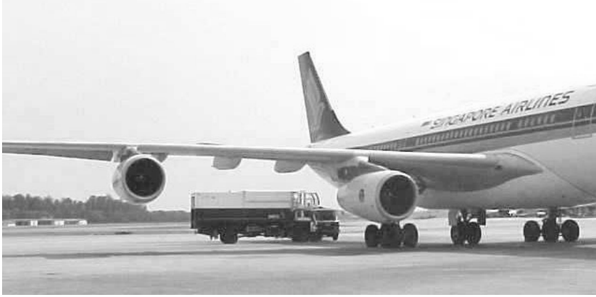
Figure 2.13. An aircraft wing can be idealized as a plate structure.
