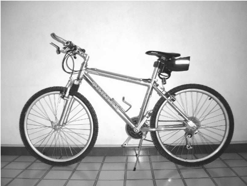
Figure 6.7. Diamond-shaped bicycle frame.
