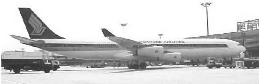
Figure 8.4. The fuselage of an aircraft can be considered to be a typical shell structure.
