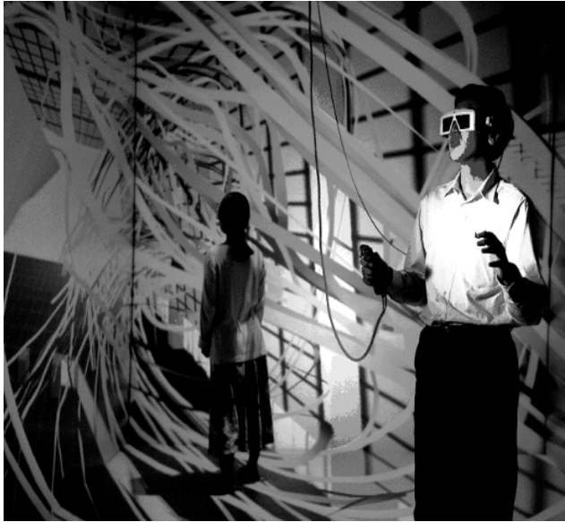
Figure 1.8. Air flow field in a virtually designed building (courtesy of the Institute of High Performance Computing).
