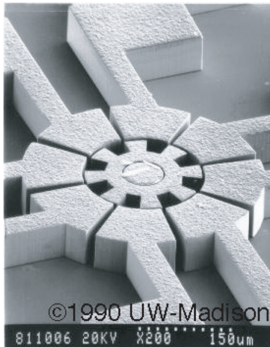
Figure 7.21. SEM image of an electrostatic micro-motor with eight rotor and 12 stator poles. (Courtesy of Professor Henry Guckel and the University of Wisconsin-Madison.)
